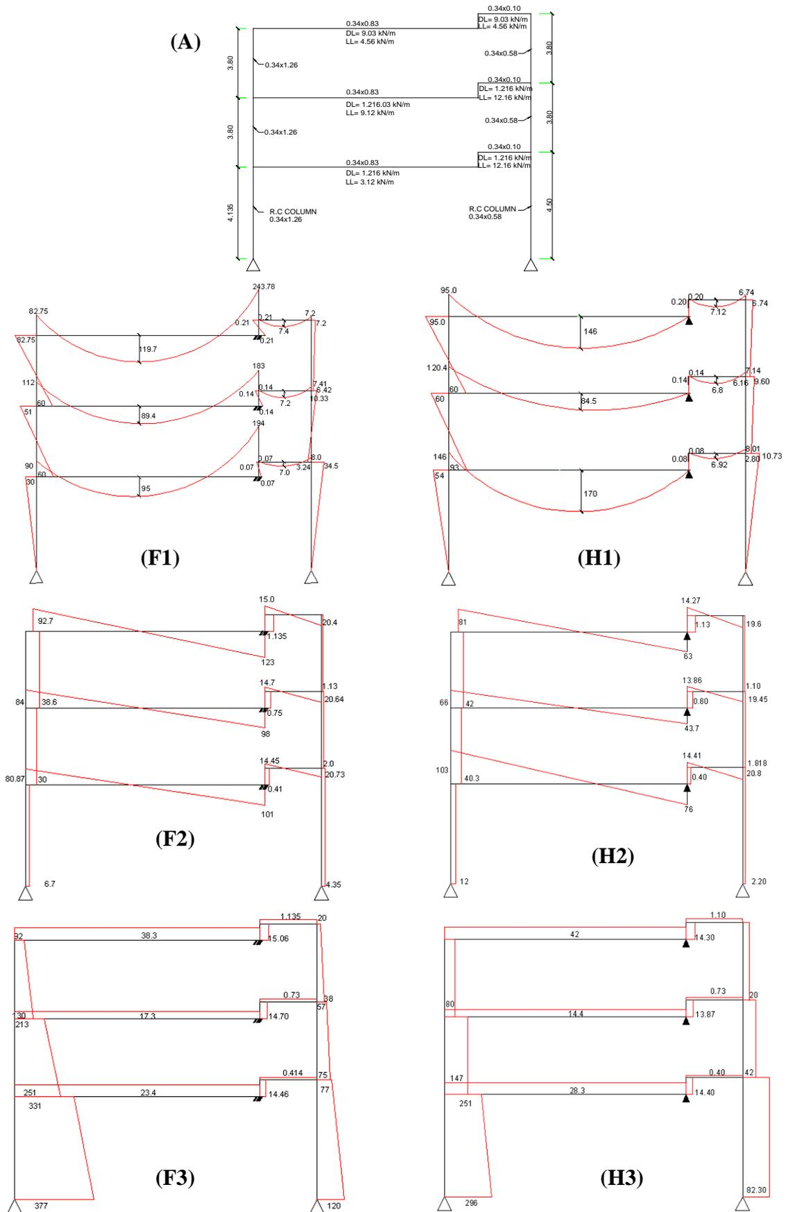
**Figure 5.** (A) Loading diagram, (F1-H1) Moments under gravity, (F2-H2) Shear forces under gravity load, (F3-H3) Axial forces under gravity load (Note: F-fixed, H-hinged)
