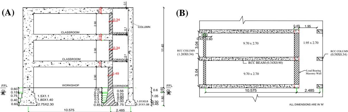
**Figure 3.** (A) Typical section through building; (B) Part plan at approximately +3.7 m level from ground level
