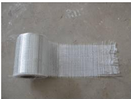
Figure 2.1. Uniaxial fabric for stripes
