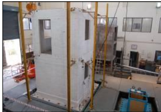
Figure 4.2. Application with quadaxial textile (west-south-side)
