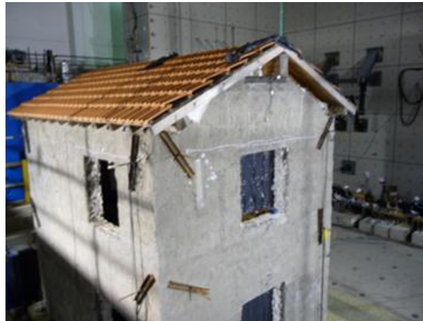
Figure 3.4. Reinforced building with quadaxial fabric
