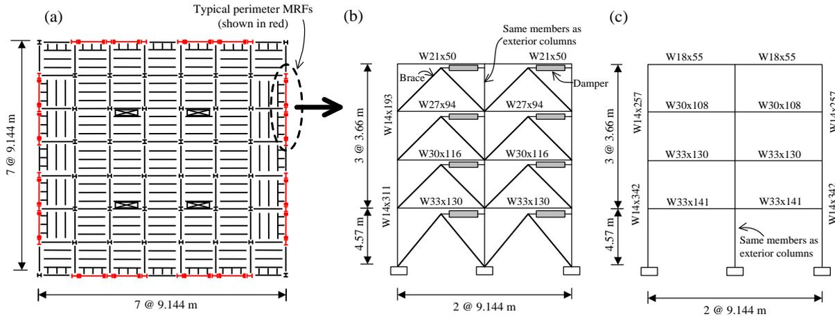
**Figure 2.** (a) Plan view of the prototype building, (b) Elevation of MRF with dampers and (c) Elevation of SMRF
