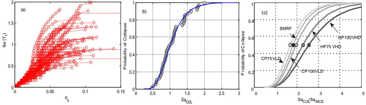
**Figure 5.** (a) Relationship between  $S_a$  and peak story drift  $\theta_s$  resulting from IDA for SMRF, (b) Cumulative distribution of  $S_{a_{COL}}$  with a fitted curve for SMRF, and (c) Fitted cumulative distribution of  $S_{a_{COL}}$  for SMRF and MRFs with dampers considered in this study
