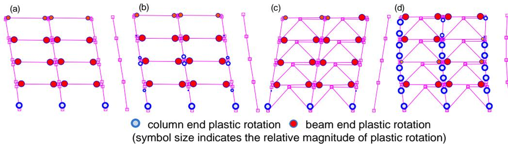
**Figure 6.** Typical incipient collapse modes (a) and (b) predicted for SMRF, and (c) and (d) predicted for MRFs with dampers.
