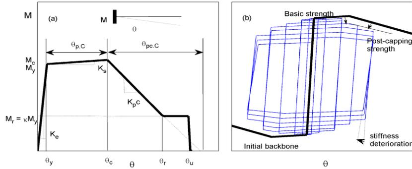
**Figure 3.** (a) Backbone curve, and (b) Cyclic moment rotation behaviour for the cyclic deterioration model
