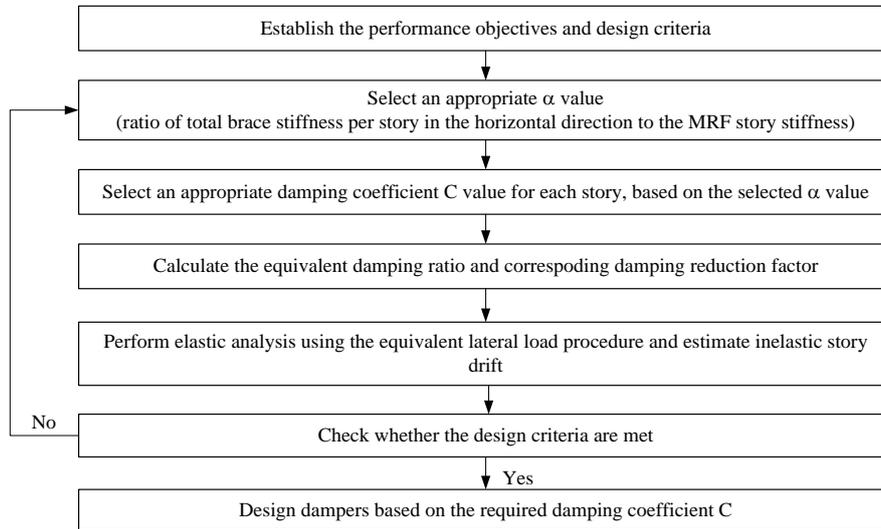
**Figure 1.** Modified simplified design procedure for MRF's with fluid viscous dampers
