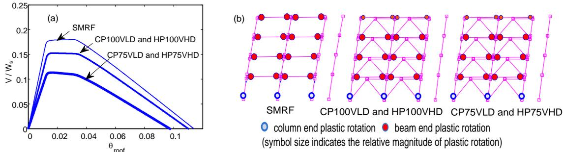
**Figure 4.** (a) Backbone curve, and (b) Cyclic moment rotation behaviour of the of the cyclic deterioration model
