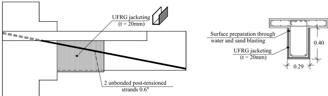
**Figure 3.3.** Detailing of the UFFG jacketing and unbonded strand post-tensioning system (specimen S3)
