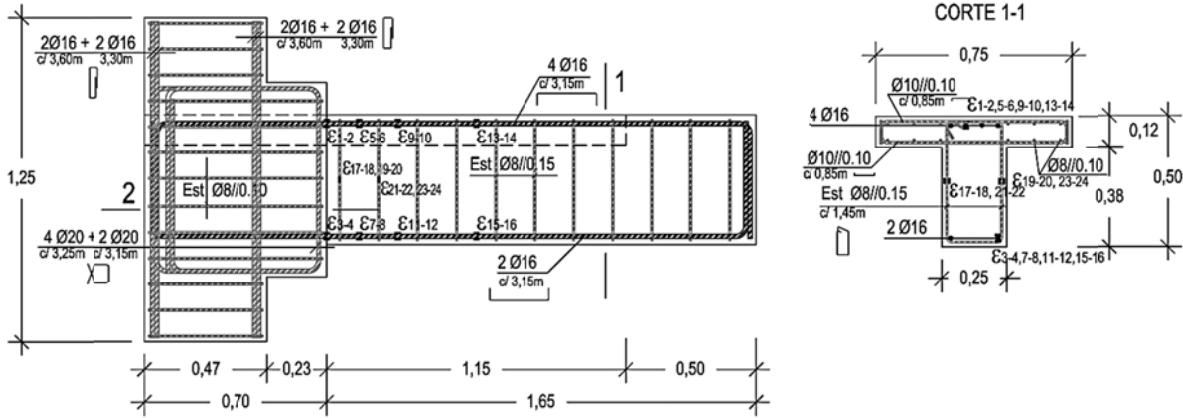
**Figure 3.1.** Geometry, detailing and internal instrumentation of the reference specimen (S1)
