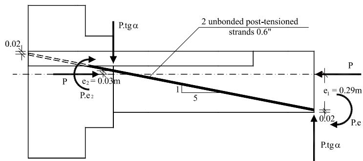
**Figure 3.2.** Detailing of the strengthening solution with unbonded post-tensioning system (specimen S2)
