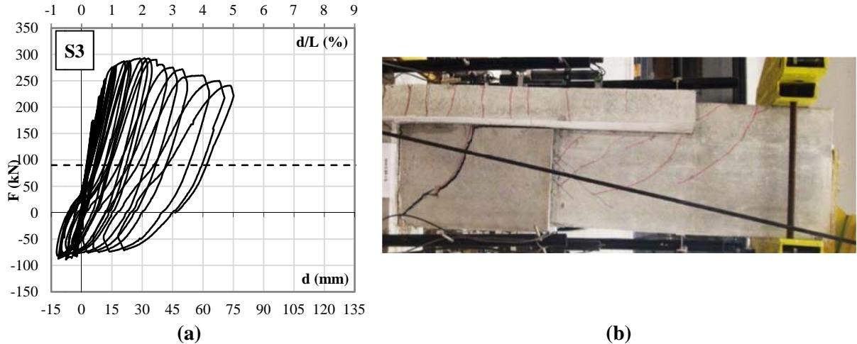
**Figure 4.3.** Specimen S3: (a) force-displacement hysteretic diagram; (b) failure mode
