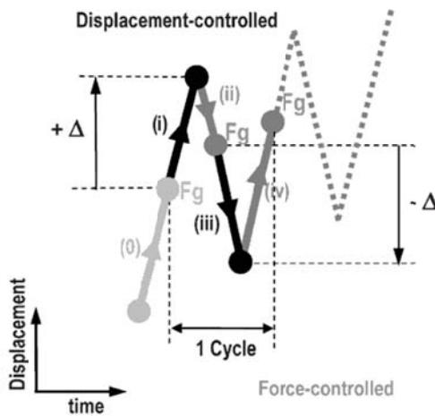
**Figure 3.5.** Typical load cycle in the test procedure [Gião et al. (2009)]
