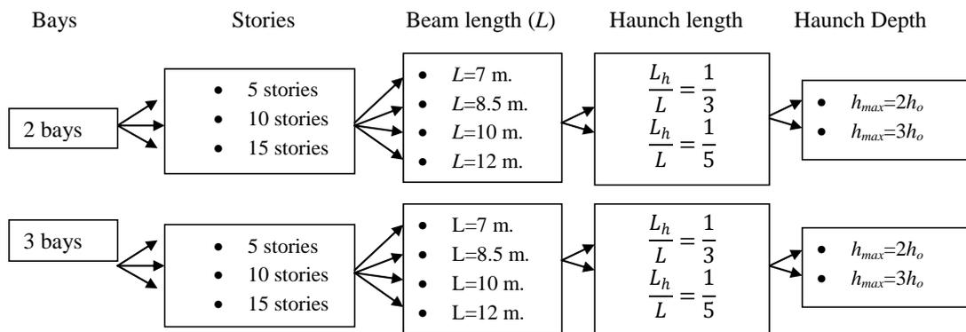
**Figure 3.2.** Summary of the conducted parametric study for the RC-MRFs with haunched beams
