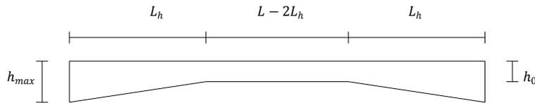
**Figure 3.3.** General geometry of the studied symmetric haunched beams
