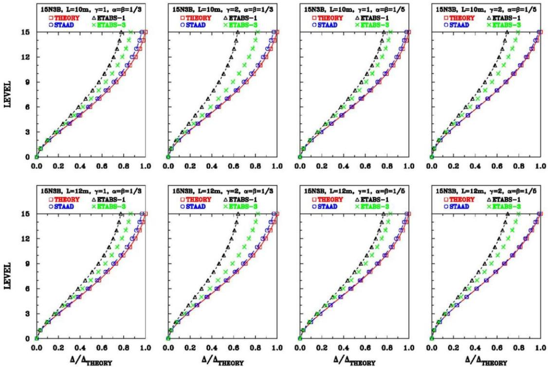
Figure 4.7. Normalized lateral displacements for fifteen-story, three-bay frames with bay widths  $L=10\text{m}$  and  $L=12\text{m}$
