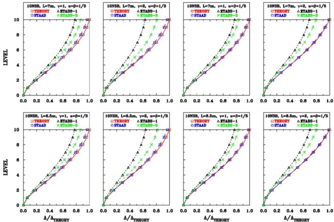
Figure 4.4. Normalized lateral displacements for ten-story, three-bay frames with bay widths  $L=7\text{m}$  and  $L=8.5\text{m}$
