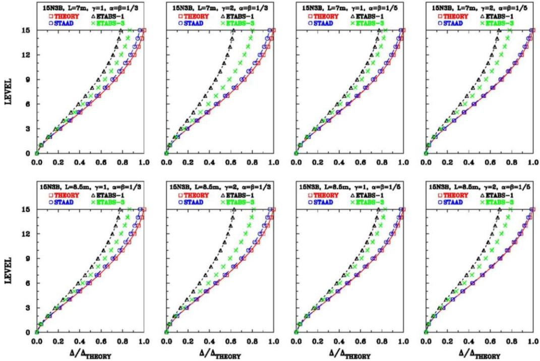
Figure 4.6. Normalized lateral displacements for fifteen-story, three-bay frames with bay widths  $L=7\text{m}$  and  $L=8.5\text{m}$
