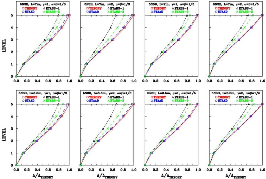
Figure 4.2. Normalized lateral displacements for five-story, three-bay frames with bay widths  $L=7m$  and  $L=8.5m$
