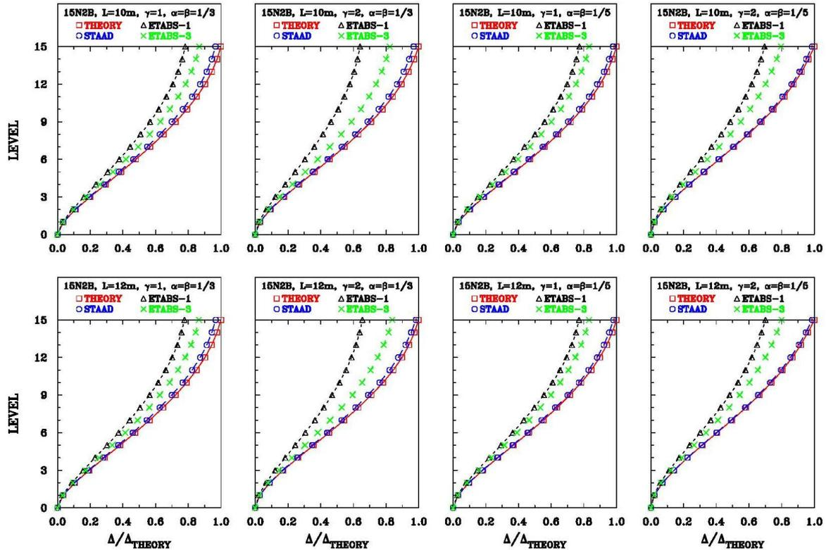
Figure 4.8. Normalized lateral displacements for fifteen-story, two-bay frames with bay widths  $L=10\text{m}$  and  $L=12\text{m}$
