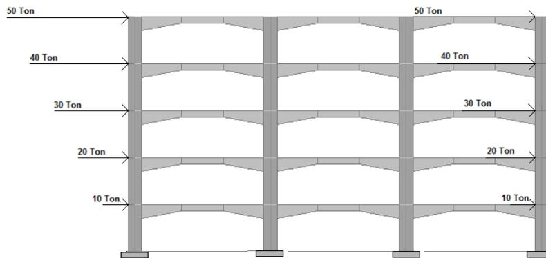
**Figure 4.1.** Applied lateral loads for the five-story models
