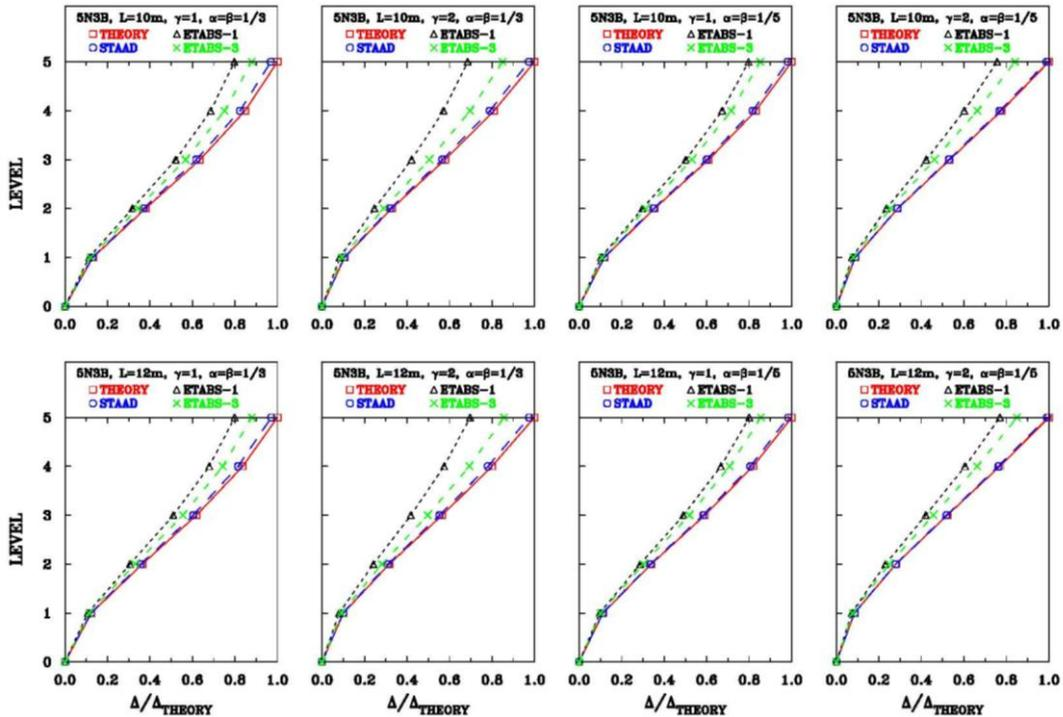
Figure 4.3 Normalized lateral displacements for five-story, three-bay frames with bay widths  $L=10m$  and  $L=12m$
