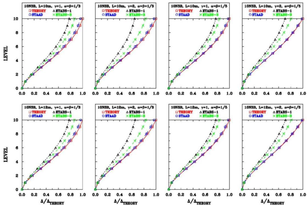
Figure 4.5. Normalized lateral displacements for ten-story, three-bay frames with bay widths  $L=10\text{m}$  and  $L=12\text{m}$
