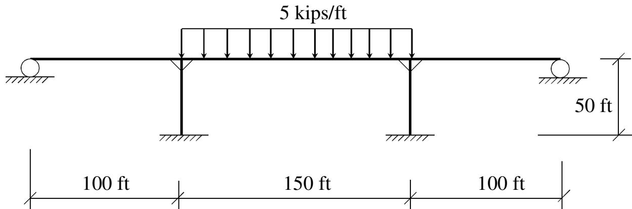
Figure 3.1. Bridge frame for example
