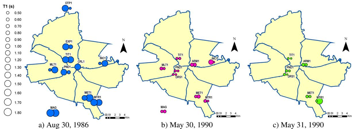
**Figure 4.3.** Bucharest: maps of the period corresponding to maximum PSD,  $T_{I(PSD)}$ , for the 1986 and 1990 earthquakes
