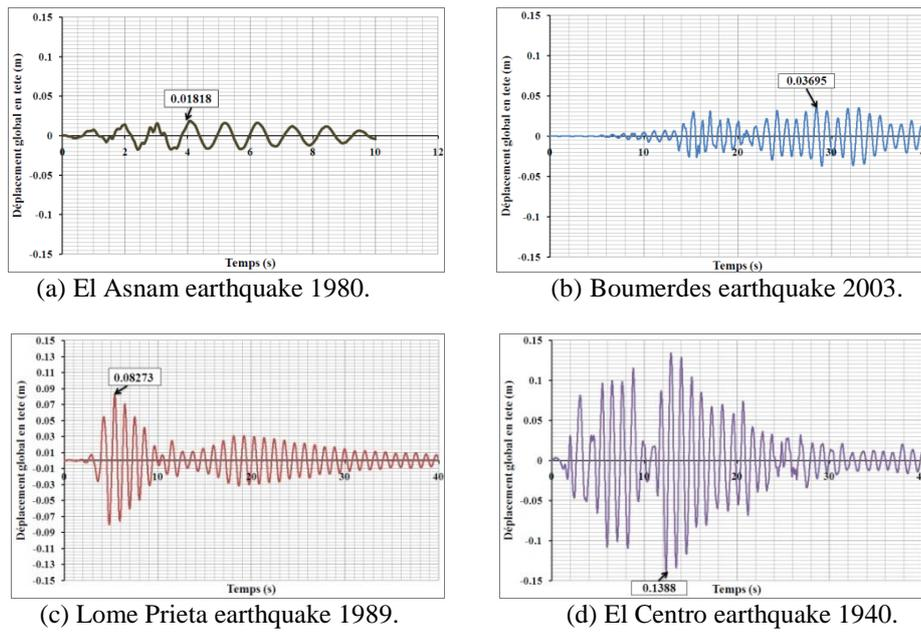
Figure 5.2. Global displacement at the top of the structure in function of time
