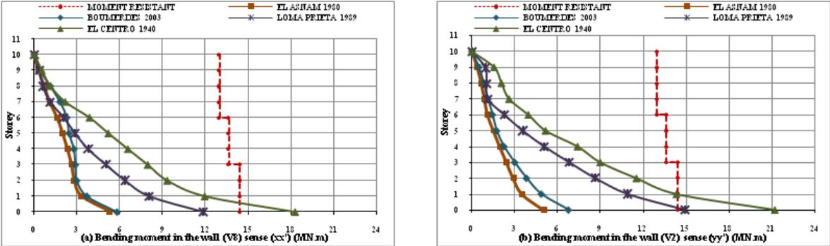
Figure 5.4. Bending moment for each floor of the structure
