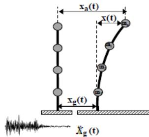
**Figure 3.1.** Schematic representation of the oscillator under seismic excitation
