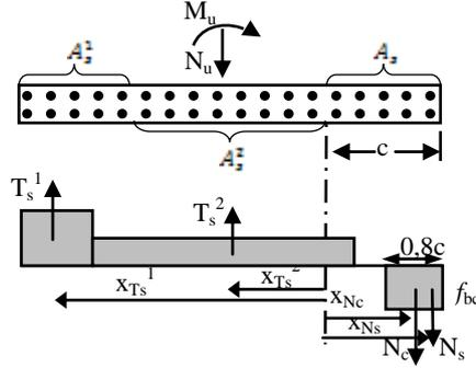
**Figure 2.3.** Behavior of a shear wall section under the different stresses
