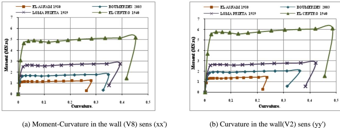
Figure 5.6. Moment-curvature diagram
