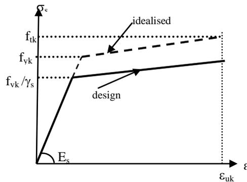
**Figure 2.2.** Stress - Strain diagram of steel for Eurocode 2 (Eurocode2, 2004)
