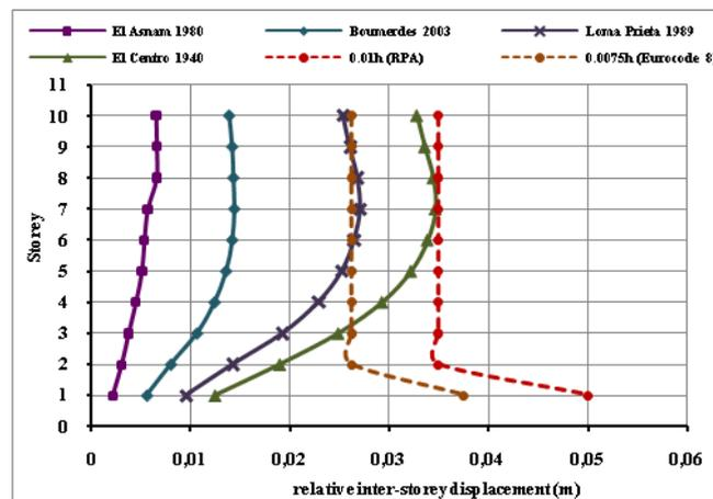
**Figure 5.1.** Inter-storey displacement of structure
