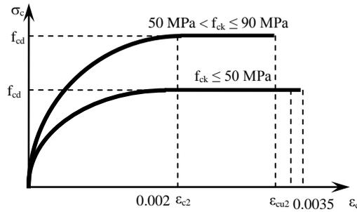
**Figure 2.1.** Stress - Strain diagram of unconfined concrete for (Eurocode2, 2004)
