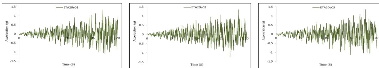
**Figure 2.** A typical ET accelerograms (ETA20e01-03)
