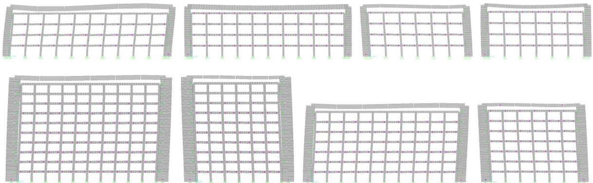
**Figure 6.** View of the plastic hinge for retrofitting frame members obtained by endurance time, dynamic time history and pushover analysis
