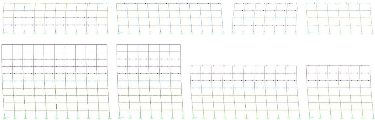
**Figure 5.** View of the plastic hinge for weak frame members obtained by endurance time, dynamic time history and pushover analysis
