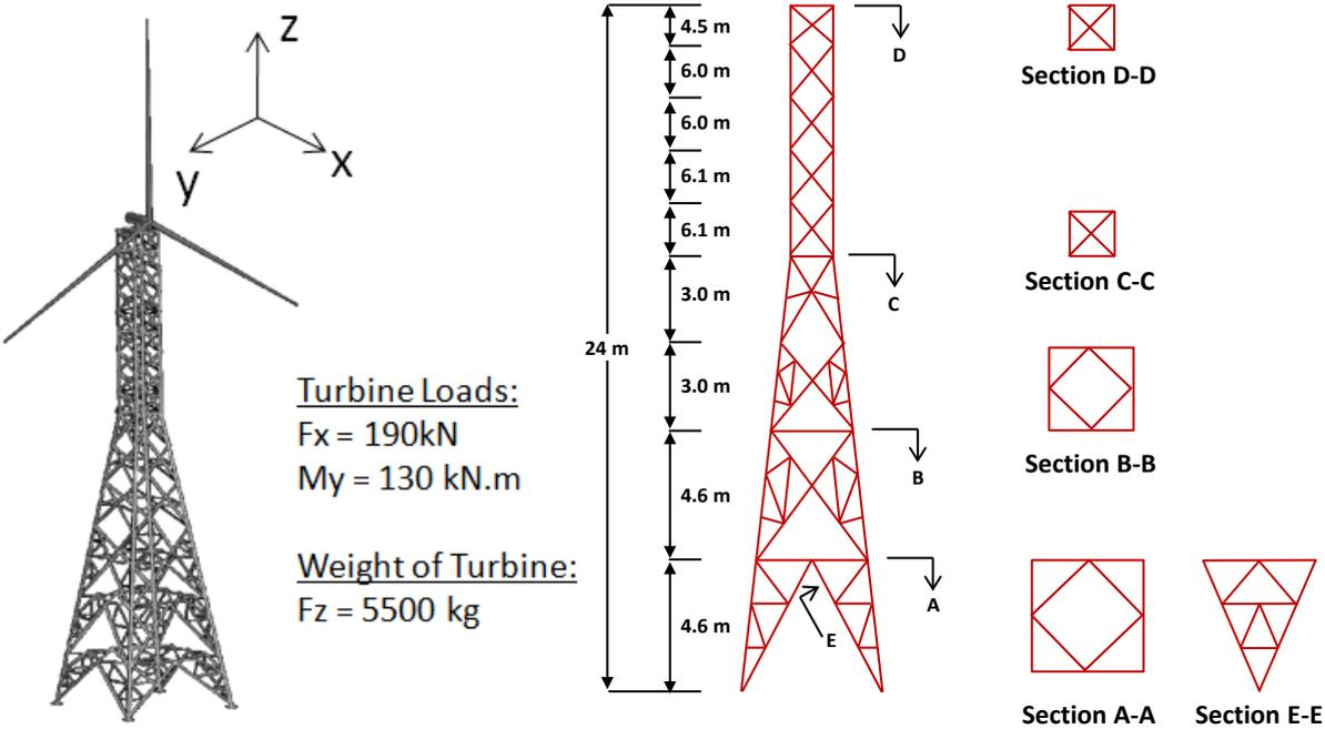
**Figure 2.1.** (Left) wind loads acting on the tower, (Right) outline drawings of the tower
