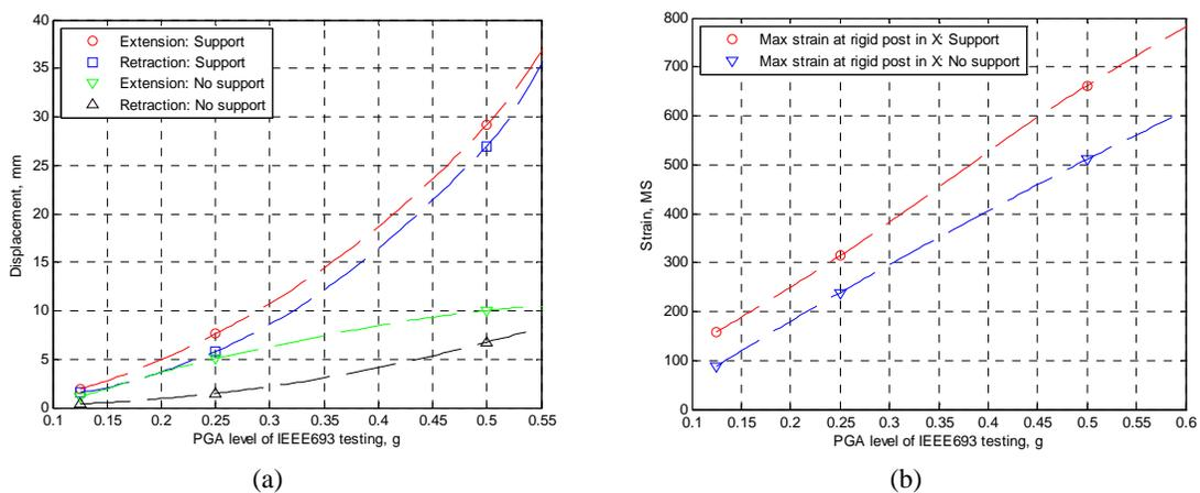
**Figure 5.** Change in distance between Rotating and Jaw posts (a) and strain at bottom section of Rigid post insulator – the most overstressed post (b)
