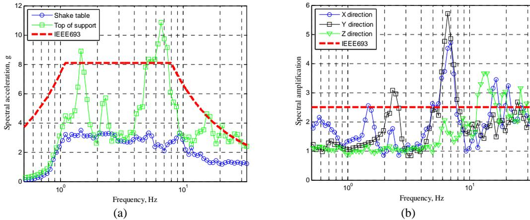
**Figure 2.** Spectral accelerations (a) and spectral ratios (b) of shake table and top of support structure
