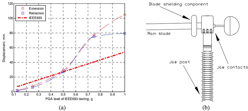
**Figure 6.** Change in distance between Rotating and Jaw posts (a) and schematic drawing of blade shielding component (b)
