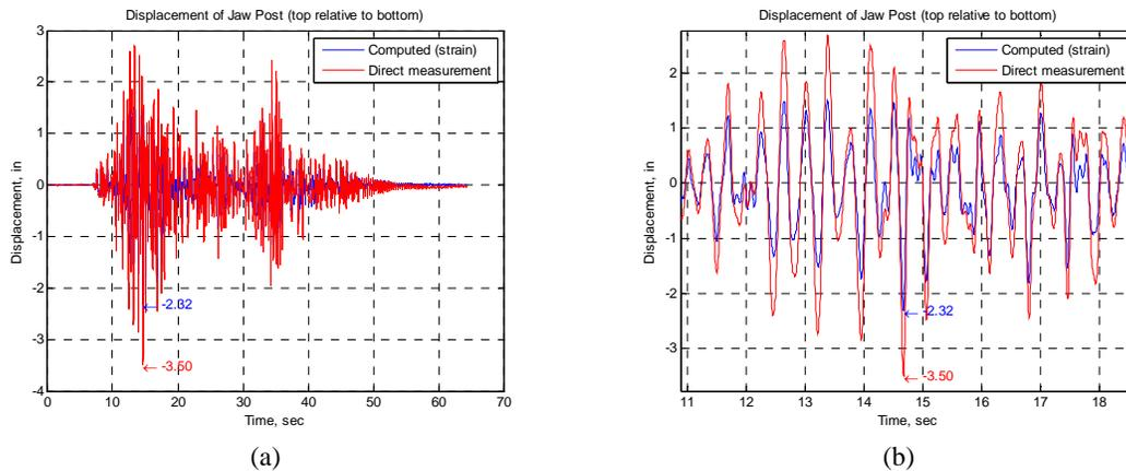
**Figure 8.** Displacement data estimated from strain versus direct measurements (a) and zoomed view of displacements in vicinity of the peak values (b)
