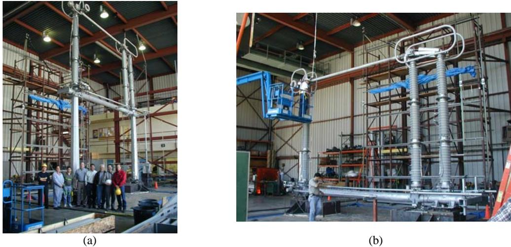
**Figure 4.** 550-kV vertical disconnect switch on 4.6 m tall support structure in closed configuration (a) and in closed configuration attached directly to a shake table platform (b).
