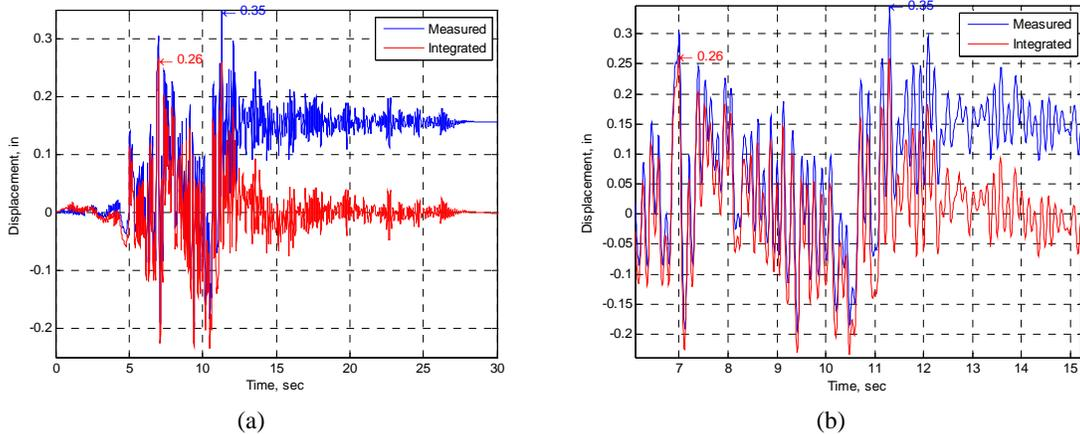
**Figure 9.** Displacement estimated from double integrated acceleration versus “directly measured” (a) and zoomed view of displacements in vicinity of the peak values (b)
