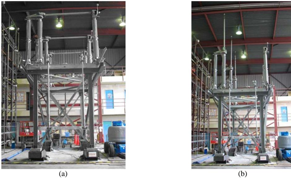
**Figure 3.** Large spectral amplifications were also observed in 230-kV switch tests: main blade closed configuration (a) and main blade open configuration (b)
