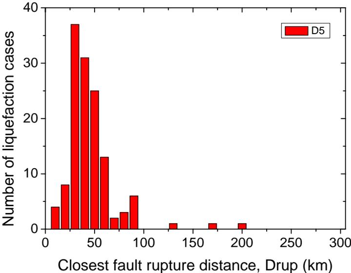
Figure 4. Number of liquefaction cases with  $D_{rup}(=D5)$
