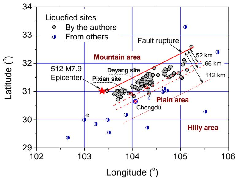
**Figure 2.** Liquefaction sites identified in the great Wenchuan earthquake
