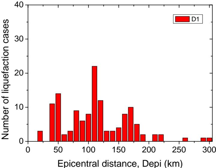
Figure 5. Number of liquefaction cases with  $D_{hyp}(=D1)$
