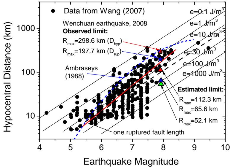
**Figure 6.** Global dataset of documented liquefaction (adapted from Wang 2007)
