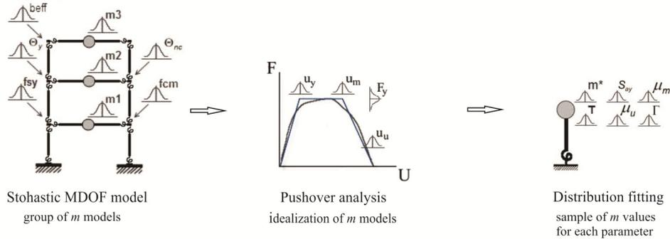
**Figure 2.1.** Schematic representation of the first step of the proposed methodology
