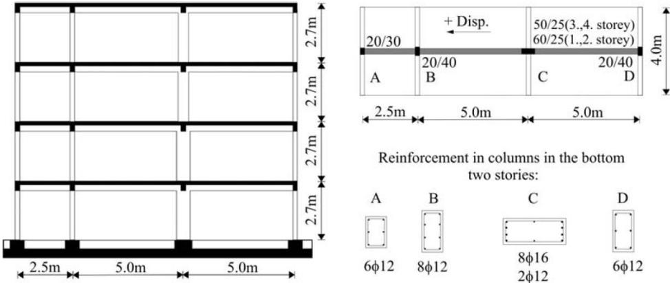
Figure 3.1. The elevation, plan view, and typical reinforcement in columns of four-storey RC frame
