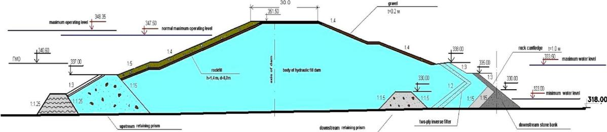
Figure 2.1. Typical Cross-Section of the Dam
