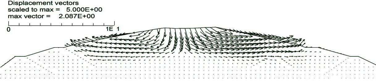
Figure 3.2. Permanent Deformation Vectors (OBE)
