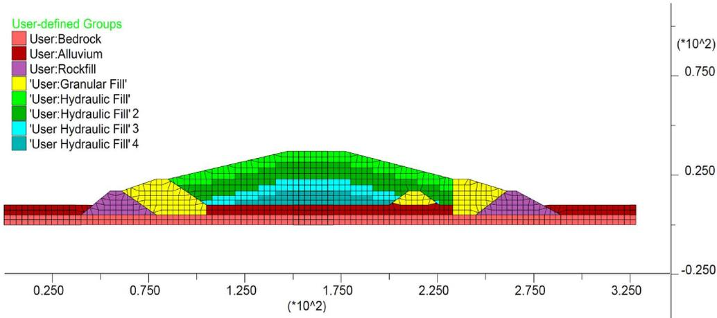
Figure 2.2. Finite Difference Grid
