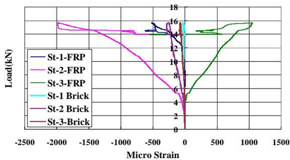
(e) Strain distribution of CFRP retrofitted wallet
