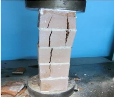
(f) Crack patterns of masonry prisms
