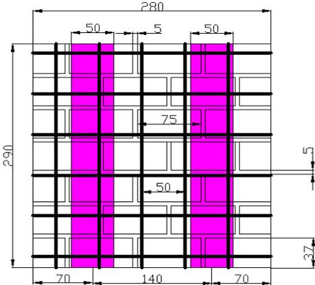
(c) Details of CFRP+PP-band retrofitted wallet
