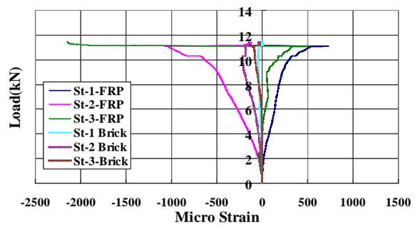
(f) Strain distribution of CFRP+PP-band retrofitted wallet
