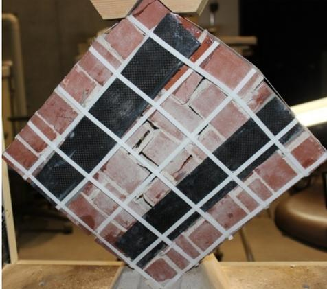
(d) Debonding failure and crack patterns of CFRP+PP retrofitted wallet
