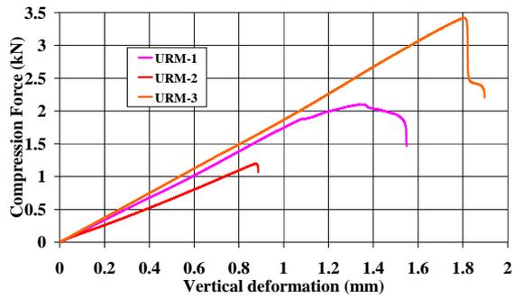
(a) Load-displacement curves of non-retrofitted wallets
