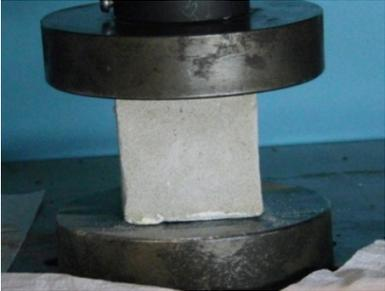
(b) Setup of mortar cube compression test
