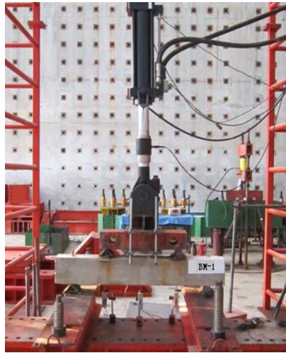
Figure 2. Test setup and loading equipment
