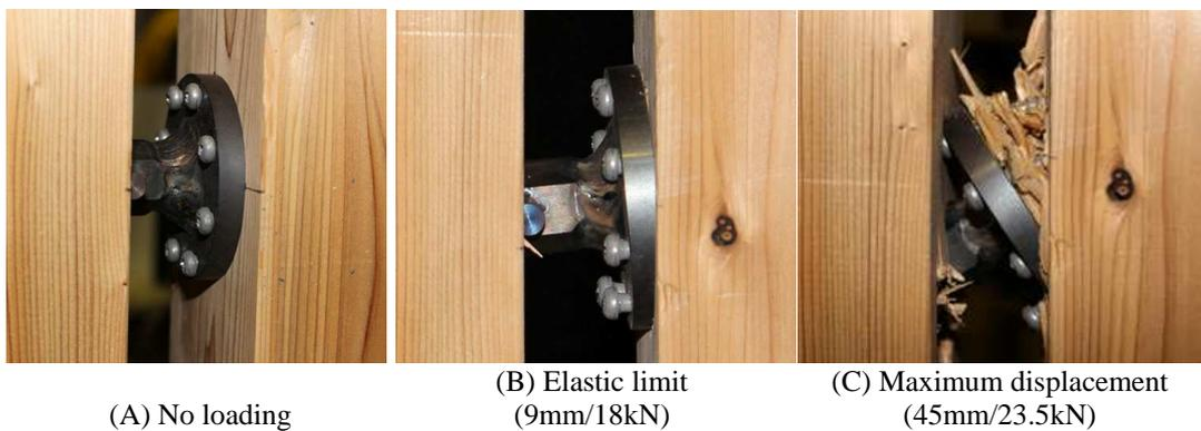
Figure 4.4. Damaged connection during the test
