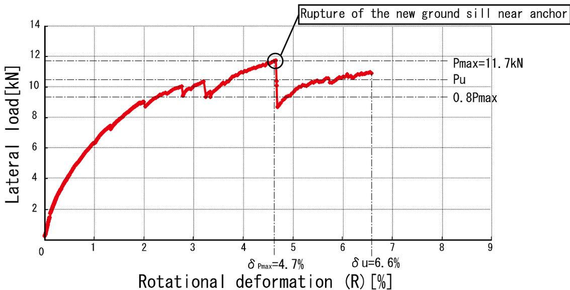
**Figure 5.2.** Envelope of the lateral load-displacement relationships
