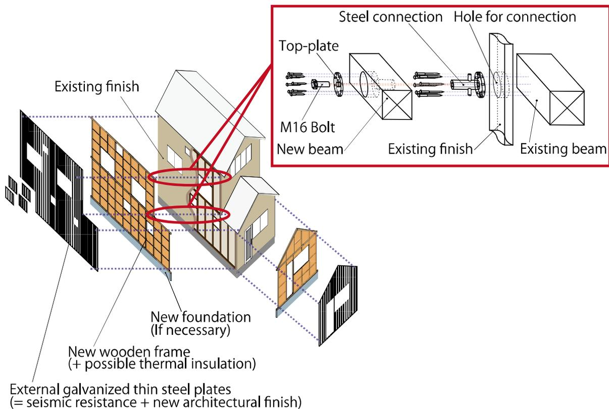
**Figure 2.1.** Composition of the reinforcing method
