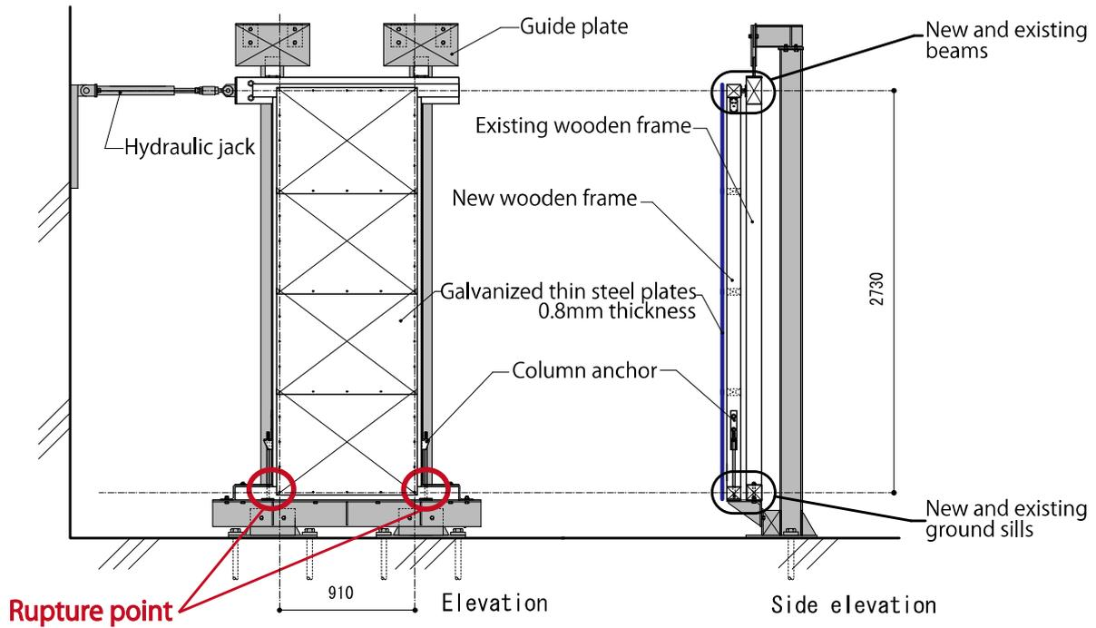
**Figure 5.1.** Specimen of shear wall test
