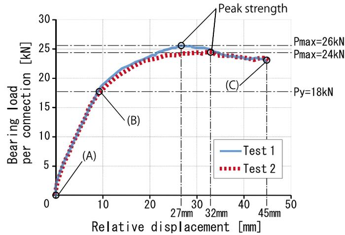
Figure 4.3. Load-displacement relationships
