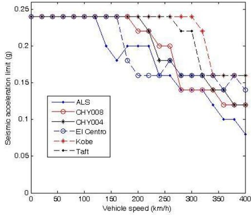
**Figure 3.** Limit values of seismic intensity determined by derailment coefficient
