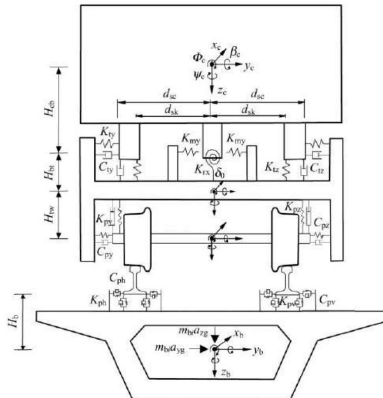
**Figure 1.** Dynamical model of train-track-bridge coupling system
