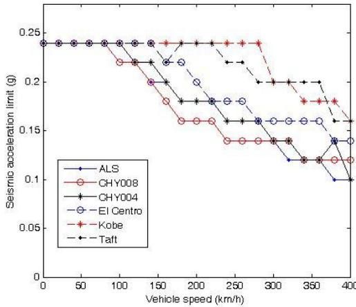
**Figure 5.** Limit values of seismic intensity determined by lateral wheel-rail force
