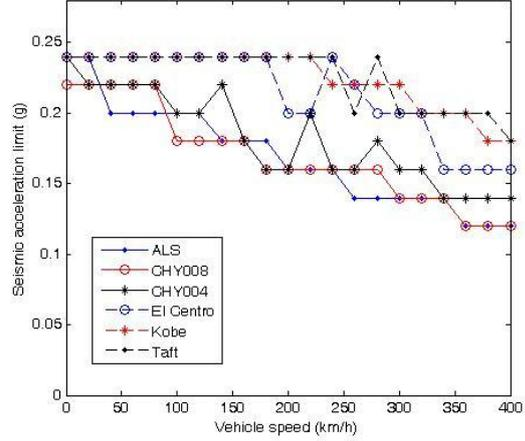
**Figure 4.** Limit values of seismic intensity determined by vehicle-body horizontal acceleration
