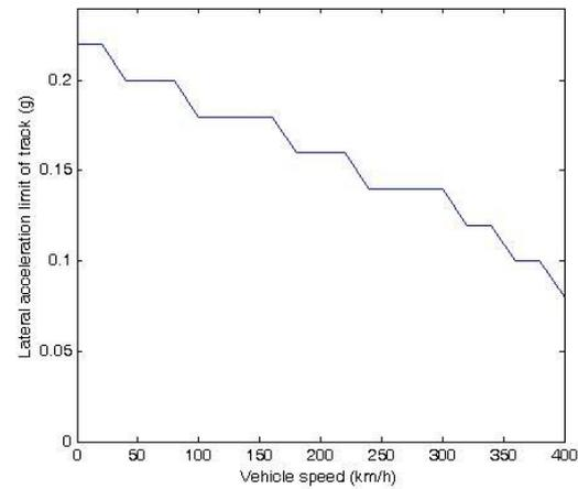
**Figure 6.** Limit values of lateral acceleration of tracks at different speed
