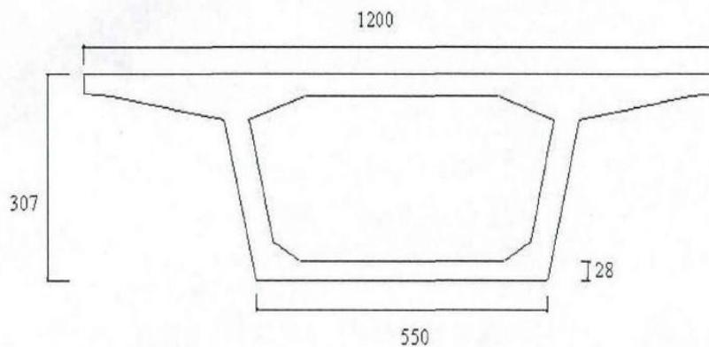
**Figure 2.** Beam section of the bridge
