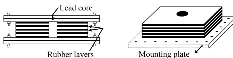
**Figure 1.1:** Lead Rubber Bearings.
