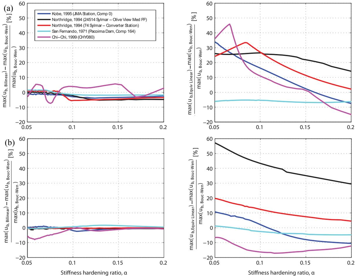
**Figure 3.1.** Relative errors of the maximum relative displacements at the isolation level considering the proposed bilinear and the corresponding equivalent linear model, varying  $\alpha$ , under the selected earthquake excitations, scaled to a (a) PGA = 0.4g and (b) PGA = 0.8g.
