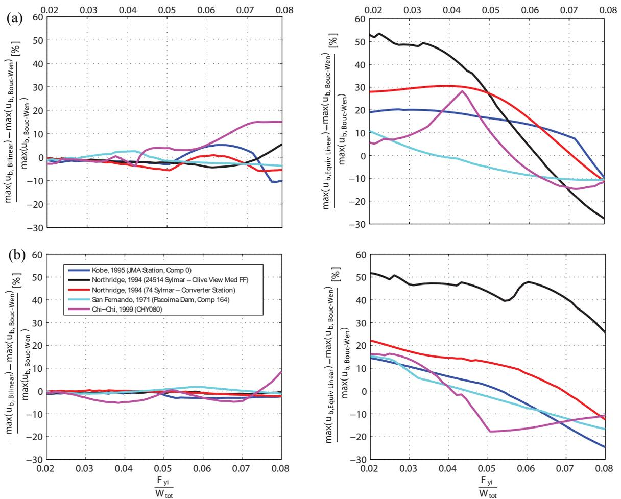
**Figure 3.3.** Relative errors of the maximum relative displacements at the isolation level considering the proposed bilinear and the corresponding equivalent linear model, varying  $F_{yi}/W_{tot}$  ratio, under the selected earthquake excitations, scaled to a (a) PGA = 0.4g and (b) PGA = 0.8g.
