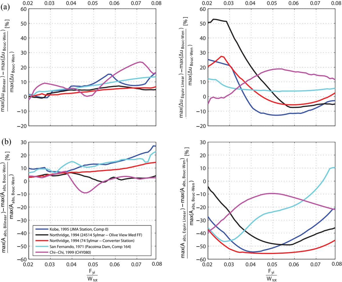
**Figure 3.4.** Relative errors of (a) the maximum interstory deflections, (b) the peak absolute floor accelerations considering the proposed bilinear and the corresponding equivalent linear model, varying  $F_{yi}/W_{tot}$  ratio, under the selected earthquake excitations, scaled to a  $PGA = 0.4g$ .
