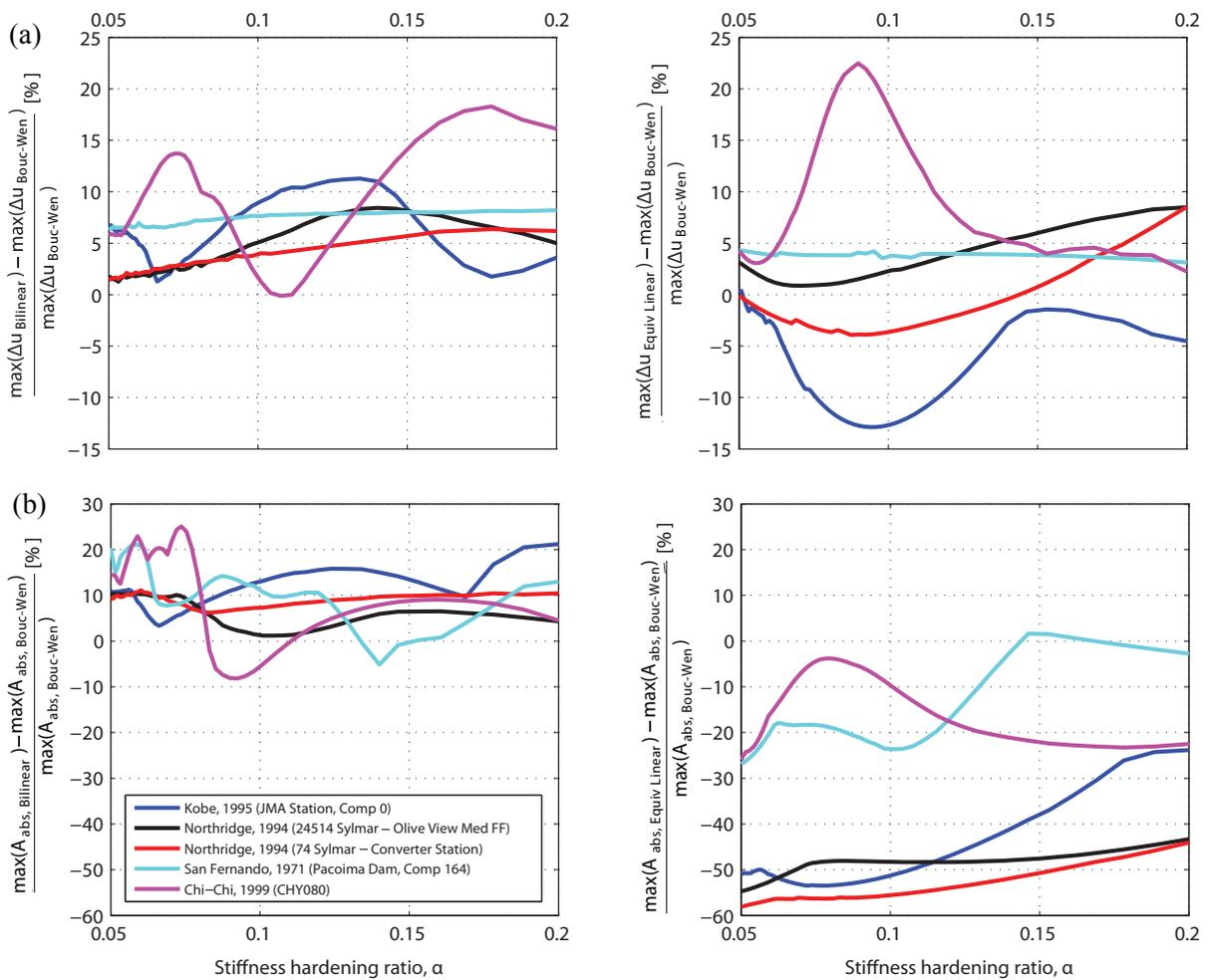
**Figure 3.2.** Relative errors of (a) the maximum interstory deflections, (b) the peak absolute floor accelerations considering the proposed bilinear and the corresponding equivalent linear model, varying  $\alpha$ , under the selected earthquake excitations, scaled to a PGA =0.4g.
