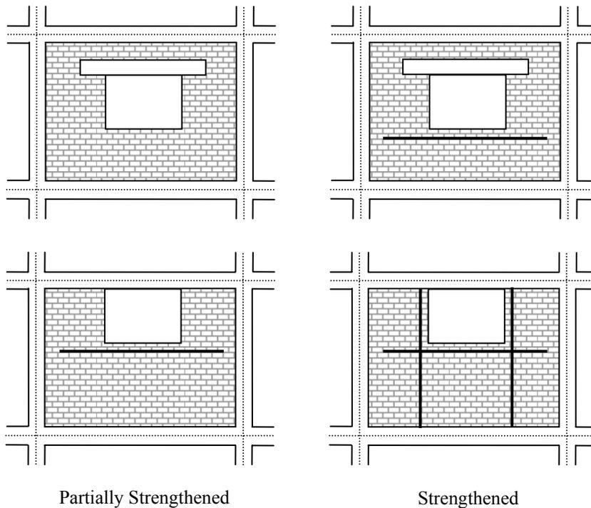
**Figure 3.2.** Examples of strengthening around opening
