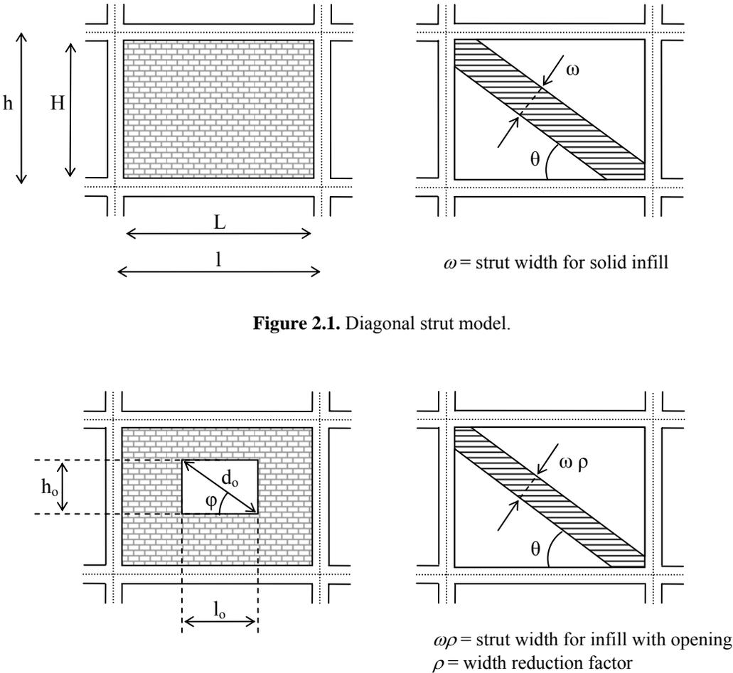
**Figure 2.1.** Diagonal strut model.
