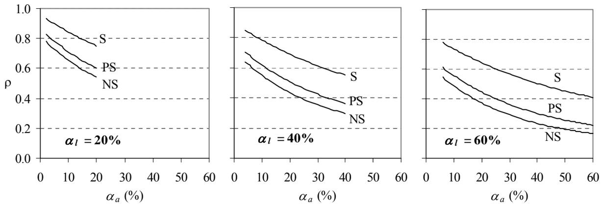
**Figure 3.5.** Proposed equations of the opening reduction factor
