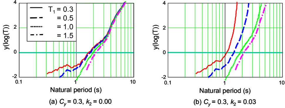
**Figure 6.** Capacity spectrum and demand spectrum in standard normal stochastic process
