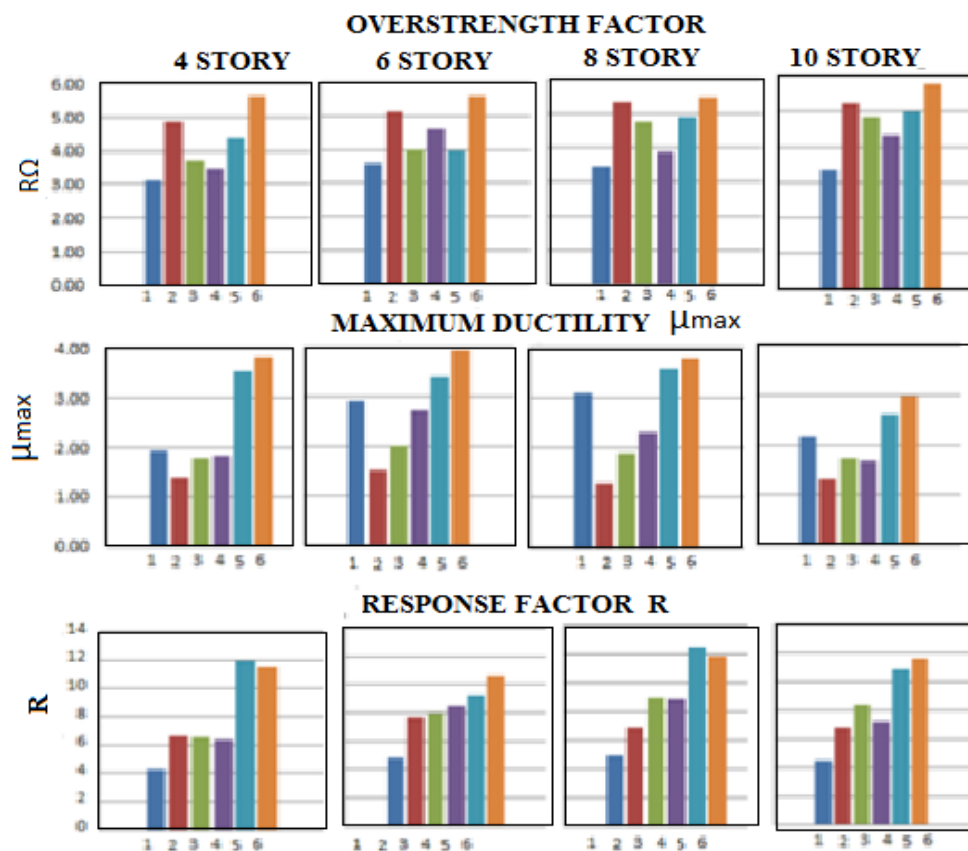
Figure 9. Values of overstrength factor, maximum ductility and response factor R
