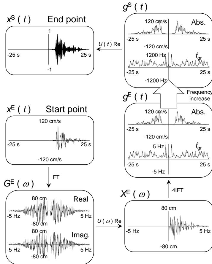
**Figure 2.2.** Flowchart of synthesis of earthquake sound waveform. “Real”, “Imag.” and “Abs.” mean real part, imaginary part and absolute value, respectively.
