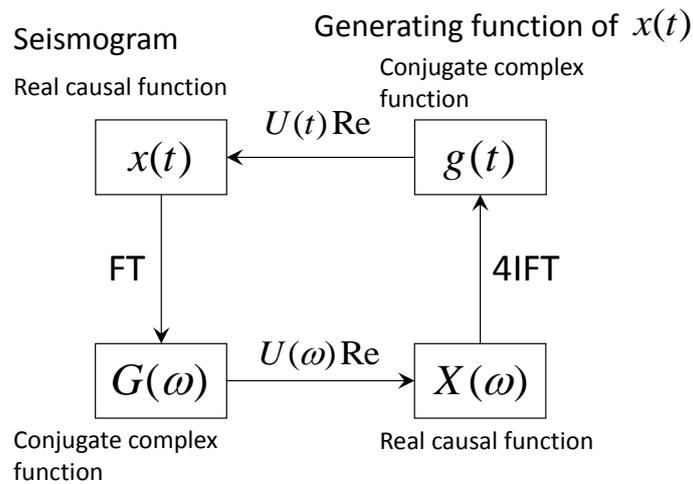
**Figure 2.1.** Schematic flow of symmetric Fourier analysis. “FT” and “IFT” mean Fourier transform and inverse Fourier transform, respectively.
