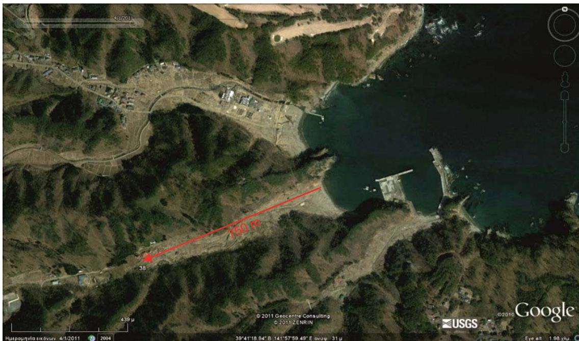
**Figure 5.** Satellite imagery before and after the 2011 Tsunami, showing the effects on coastal areas, about 5km of Miyako town, in Onatsube area. Inundation was estimated at 750m and Runup at 37m. Damage in port facilities, infrastructure, houses and industrial facilities etc., are visible, as well as effects in natural environment (Intensity: XII).
