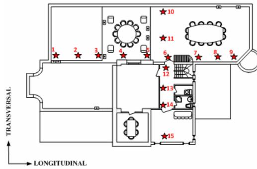
**Figure 4.** Measurement points position on level III for ambient vibration test.
