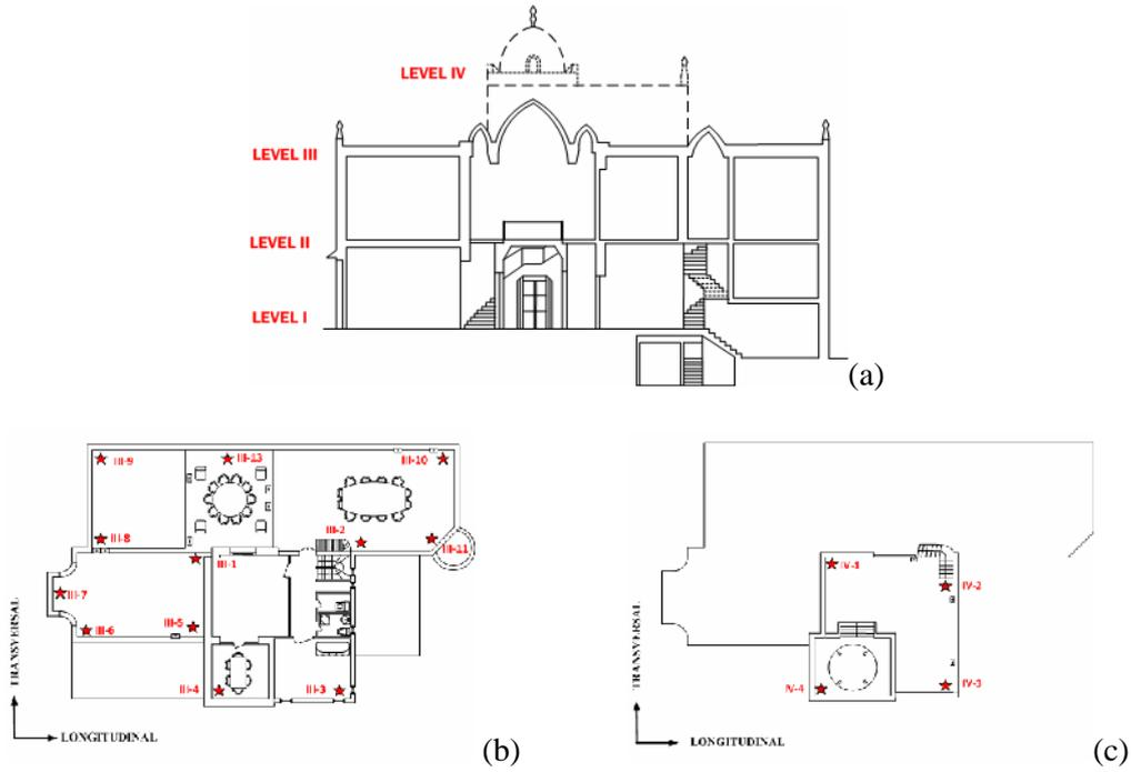
**Figure 6.** Plan view of the building and floor levels with measuring points of accelerometers:
