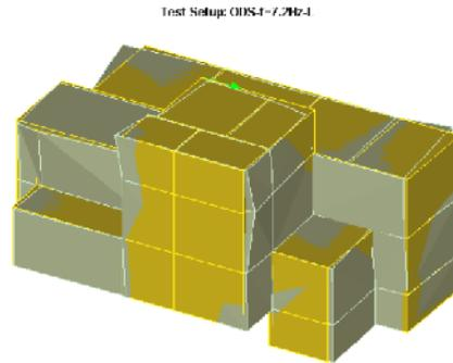
**Figure 15.** Vibration shape of the building at resonant frequency  $f=5.4\text{Hz}$  by excitation in the longitudinal direction.
