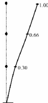
**Figure 9.** Mode shape in the longitudinal direction obtained by ambient vibration test
