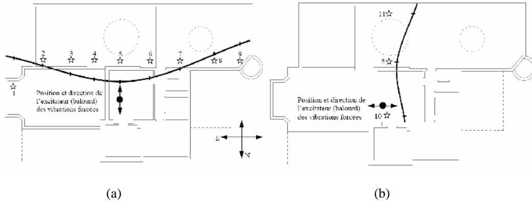
**Figure 13.** In-plan vibration mode shapes by forced vibration test (a) Transversal excitation ( $f=4.8$  Hz), (b) Longitudinal excitation ( $f=5.4$  Hz)
