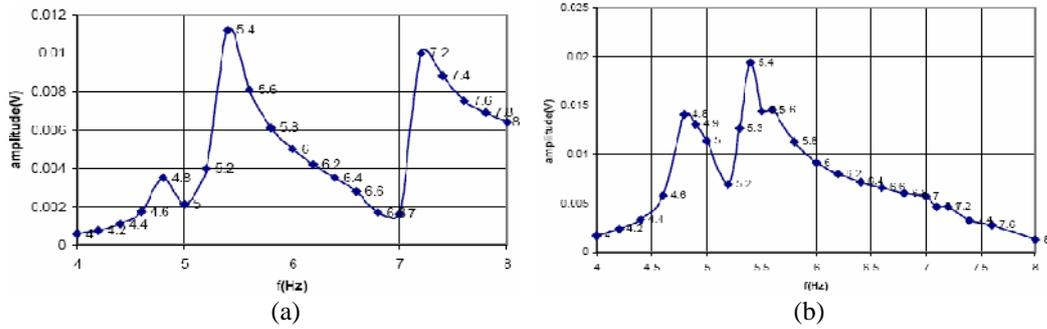
**Figure 11.** Frequency Response Curve for point III-10: (a) Transversal excitation, (b) Longitudinal excitation
