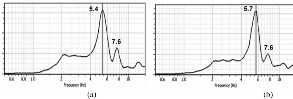
**Figure 8.** Fourier amplitude spectra after retrofitting: (a) Transversal direction (b) Longitudinal direction
