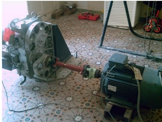
**Figure 5.** Eccentric mass shaker for excitation of harmonic force
