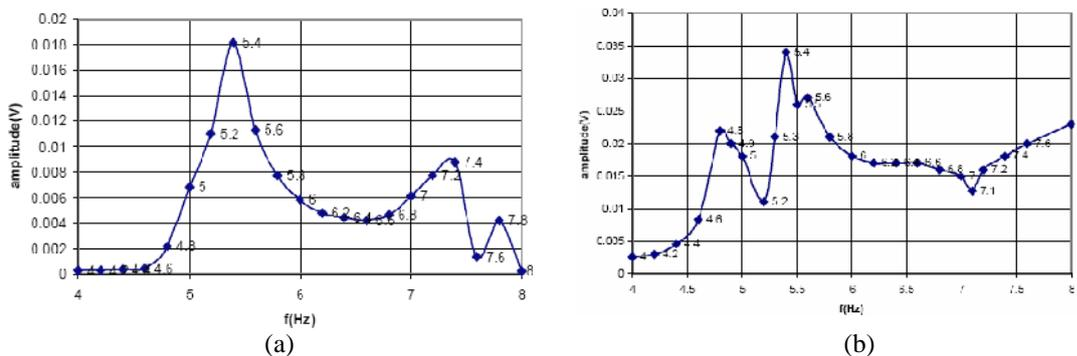
**Figure 10.** Frequency Response Curve for point III-1: (a) Transversal excitation, (b) Longitudinal excitation
