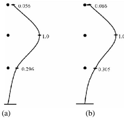
**Figure 12.** Vibration mode shapes by forced vibration test (a) Transversal excitation ( $f=4.8$  Hz), (b) Longitudinal excitation ( $f=5.4$  Hz)
