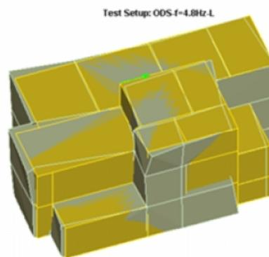
**Figure 14.** Vibration shape of the building at resonant frequency  $f=4.8$ Hz by excitation in the transversal direction.
