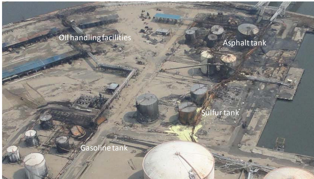
Figure 5. Burned-out section in a refinery
