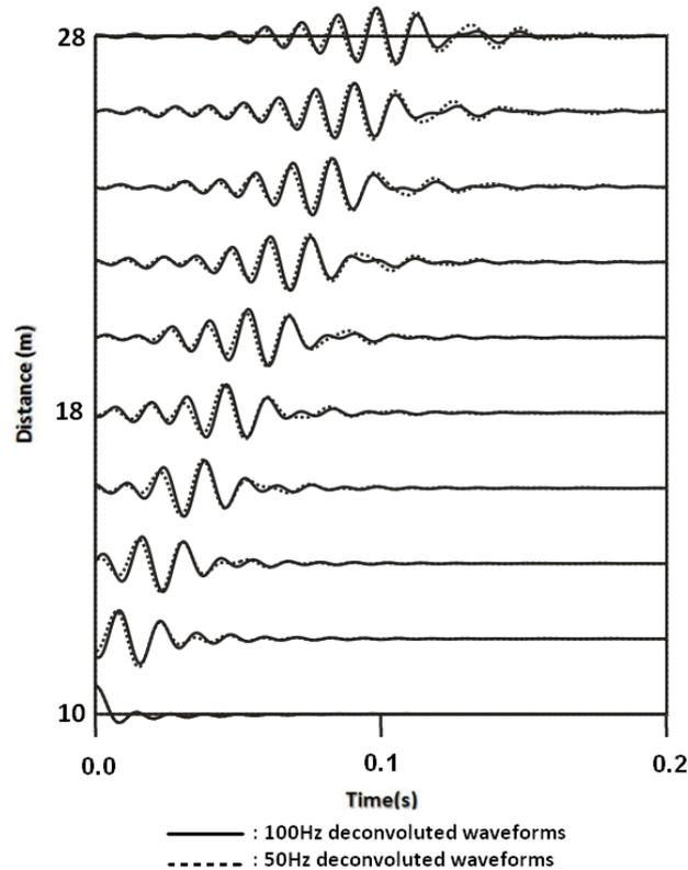
**Figure 1.** Comparing deconvoluted wave forms from different source frequencies.
