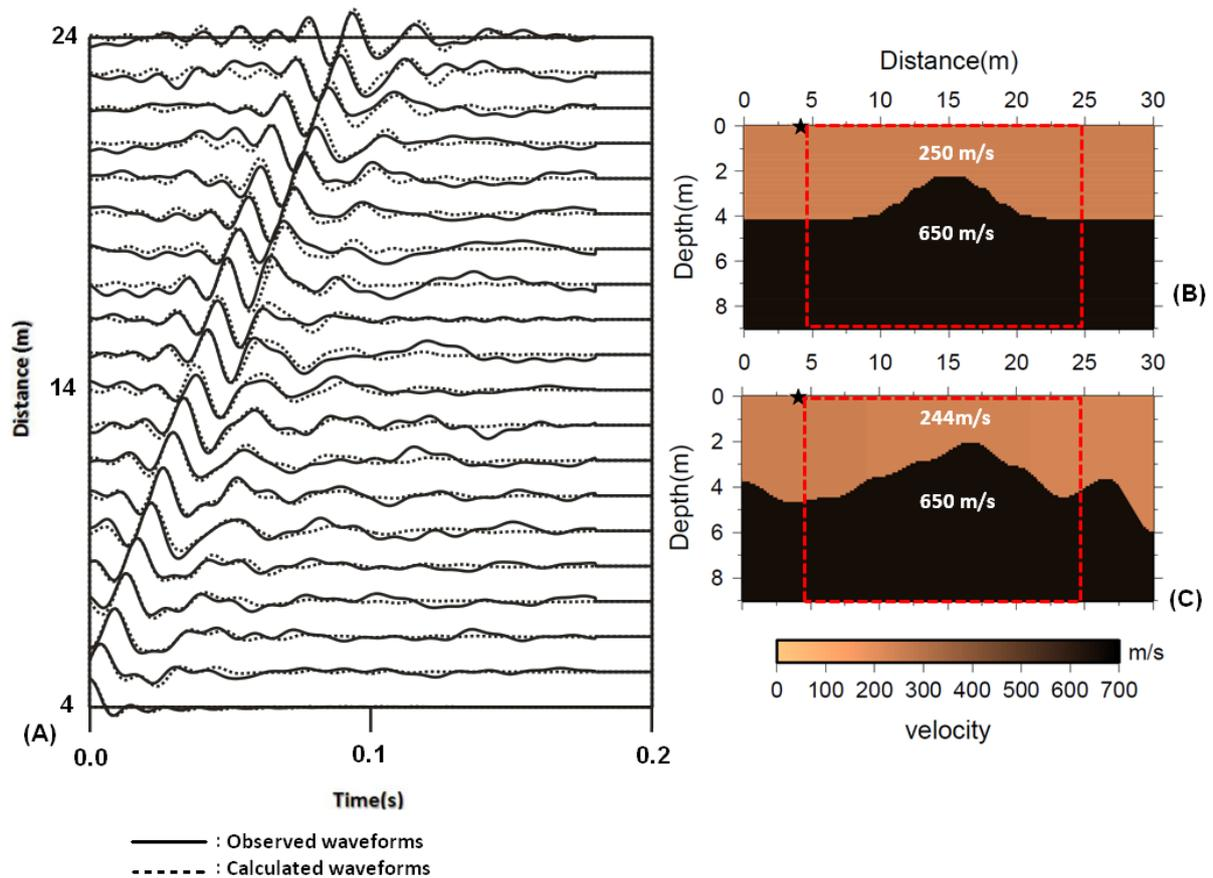
**Figure 4.** Inversion results of the two layers model with irregular interface using a noisy signal
