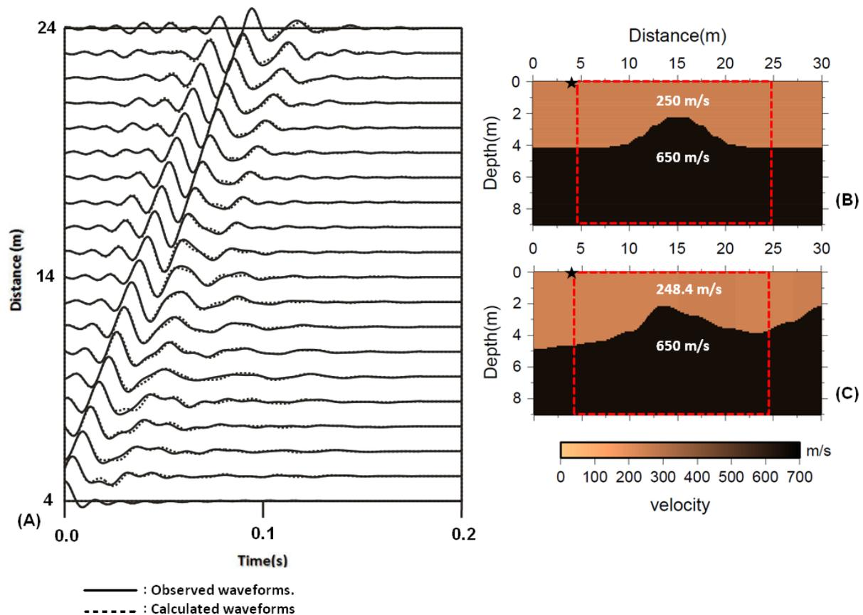
**Figure 3.** Inversion results of the two layers model with irregular interface
