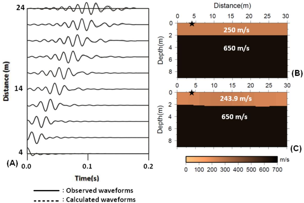
**Figure 2.** Inversion Results of the two layer flat interface soil model:
