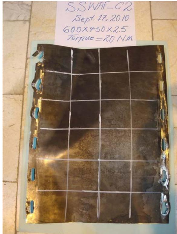
**Figure 7.** The deformed shape of one of the plates used in the second cyclic test with the severe deformations and tearing at the vicinity of the slots.
