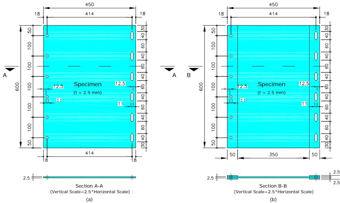
**Figure 3.** Dimensions of the specimens and the details and locations of the slots and bolt holes used in them. a) Specimen of Type 2 (see Table 1), and b) specimen of Type 3 with BSPs.
