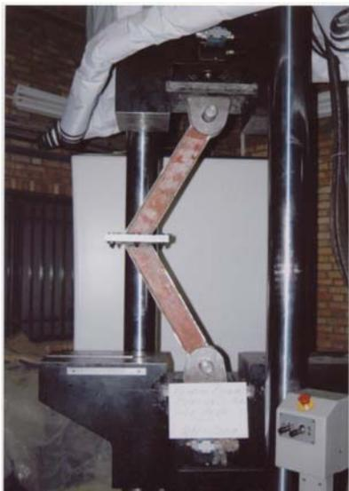
**Figure 4.** The 1st specimen, with IPE100 sections, before the test.
