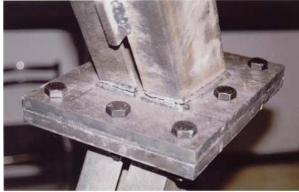
**Figure 16.** The developed cracks and the detachment of the upper segment and its endplate due to ‘lack of fusion.’
