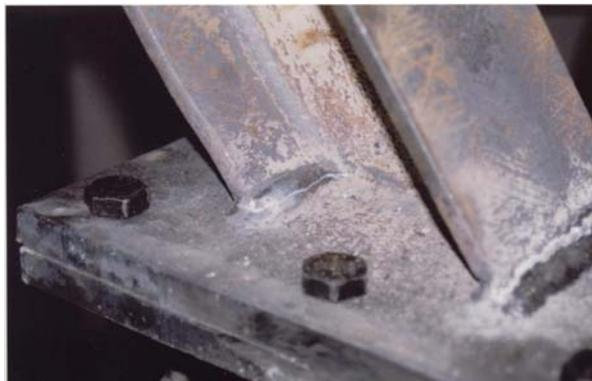
**Figure 10.** Developed cracks at the other side of the upper segment of the 2nd test assembly with HE-A100 sections.
