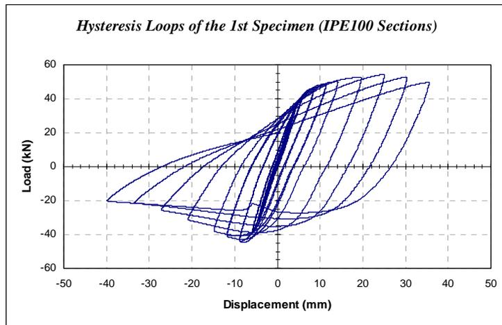
**Figure 7.** Hysteresis loops of the 1st test assembly with IPE100 sections used for the two segments of the devised Broken Beam Bracing System.
