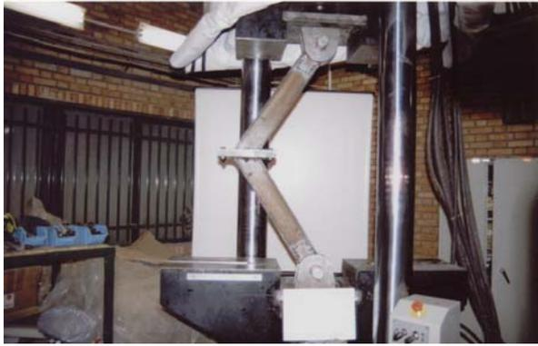
**Figure 8.** The 2nd specimen, with HE-A100 sections, before the test.
