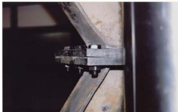
**Figure 11.** Local buckling of lower flange of the upper segment of the 2nd test assembly with HE-A100 sections.
