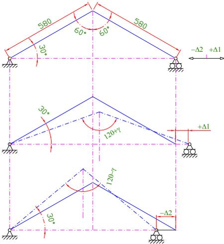
**Figure 3.** The idealized model of the bracing system subjected to linear displacements in tension ( $\Delta_1$ ) and compression ( $\Delta_2$ ) to create the rotation angles prescribed by AISC (2005) between the two segments.
