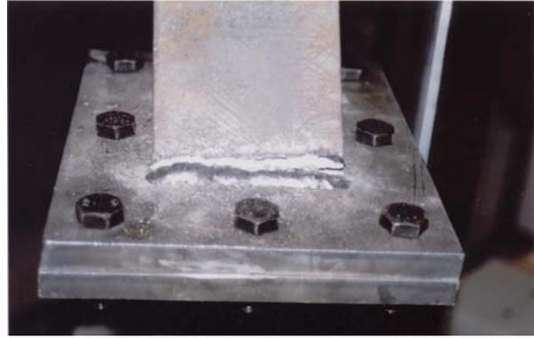
**Figure 9.** Developed cracks at the joint between the upper segment and its endplate caused by 'lack of fusion.'
