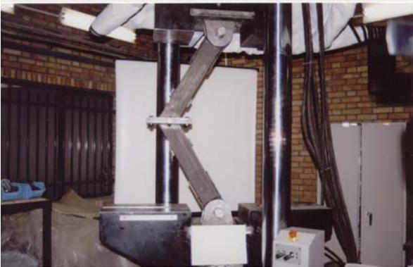
**Figure 14.** Overall front view of the 3rd specimen with 2UNP100 sections attached together with 10 mm thick battens.
