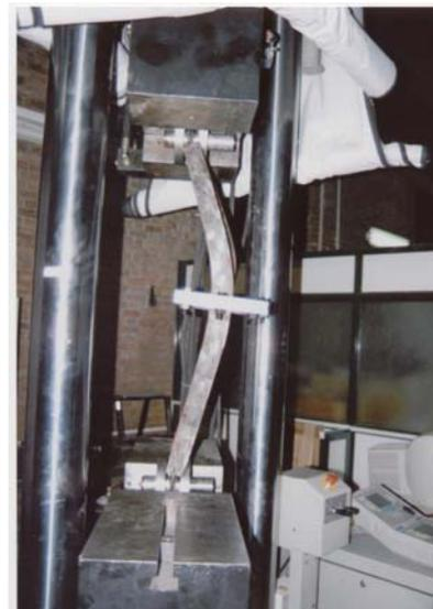
**Figure 5.** Side view of the 1st specimen at the end of the test with maximum observed out-of-plane displacements.
