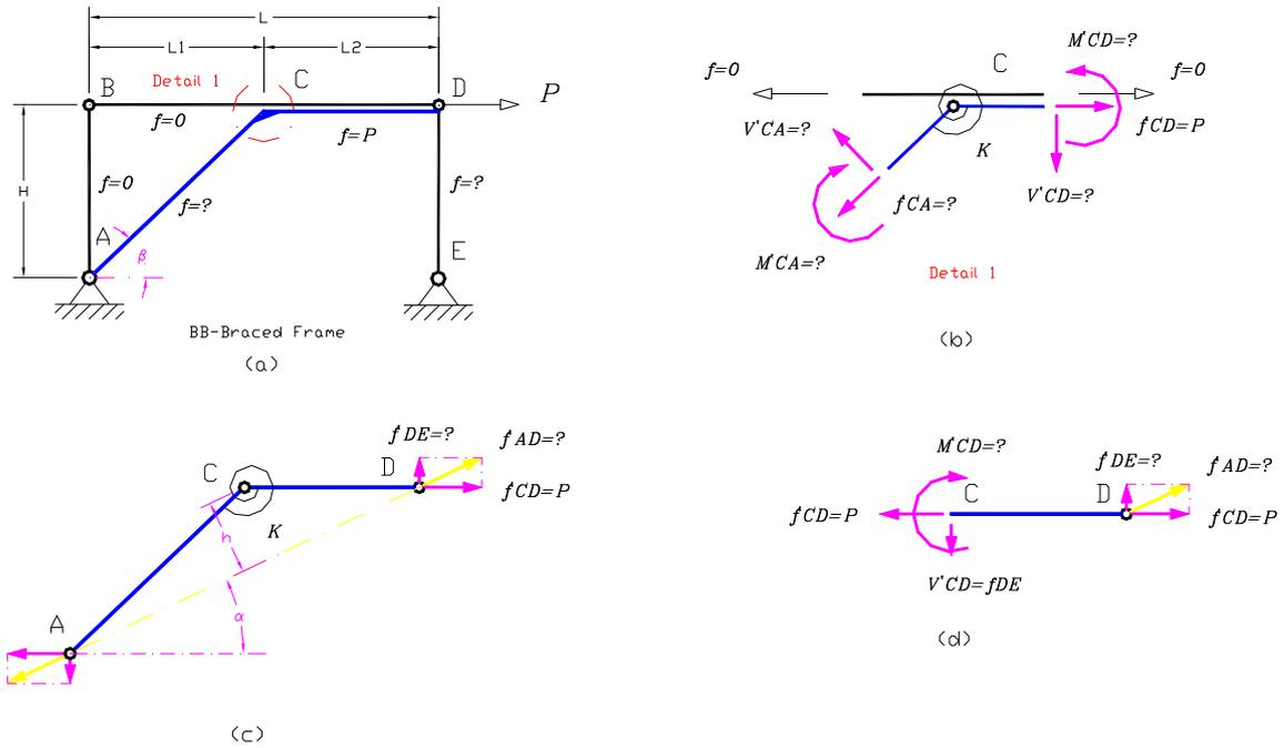
**Figure 1.** The Broken Beam Bracing System (BBBS) and its geometric and mechanical details. (a) The brace, shown in blue, fitted into a portal frame; (b) Detail 1 and the lack of physical contact between the beam and the brace; (c) the free-body diagram of the brace and the largest moment arm ( $h$ ) which leads to the maximum bending moment occurring at the brace knee; (d) free-body diagram of the horizontal segment of the brace.
