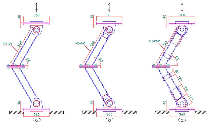
**Figure 2.** The test assemblies designed and fabricated to enable the authors to apply cyclic loading to the specimens of the bracing system. Brace segments were fabricated from (a) IPE100, (b) HE-A100, and (c) 2UNP100 sections.
