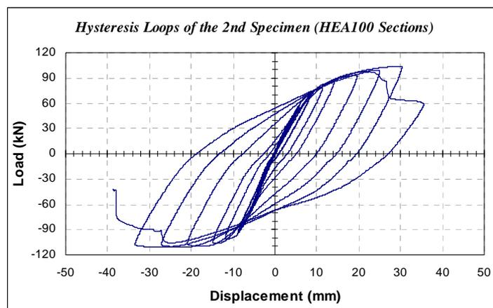
**Figure 12.** Hysteresis loops of the 2nd test assembly with HE-A100 sections used for the two segments of the devised Broken Beam Bracing System.
