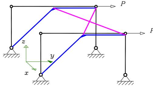
**Figure 6.** A suggested extra bracing system (in horizontal plane in magenta) to prevent the devised bracing system from having out-of-plane (lateral) deformations (buckling).
