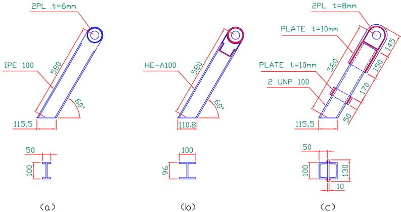
**Figure 13.** Details of the members of various test assemblies and their cross sections.
