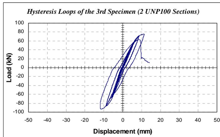
**Figure 17.** Hysteresis loops of the 3rd test assembly with 2UNP100 sections used for the two segments of the devised Broken Beam Bracing System.
