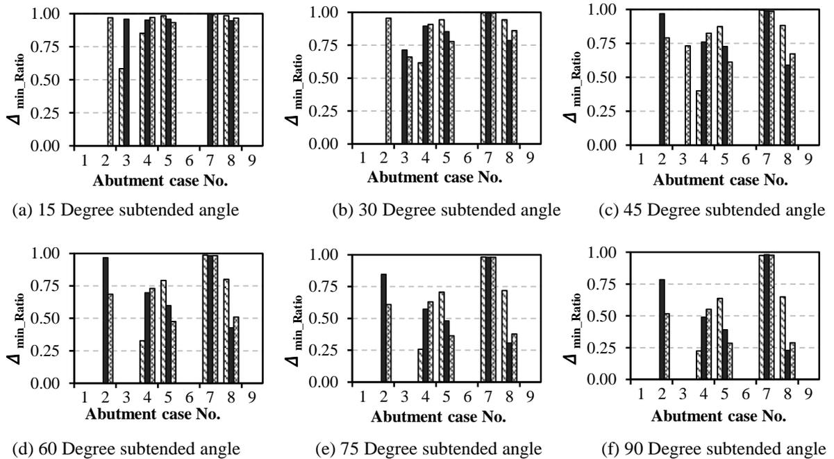
Fig. 3.6 Minimum displacement ratios of the straight to curved bridges grouped by subtended angles
