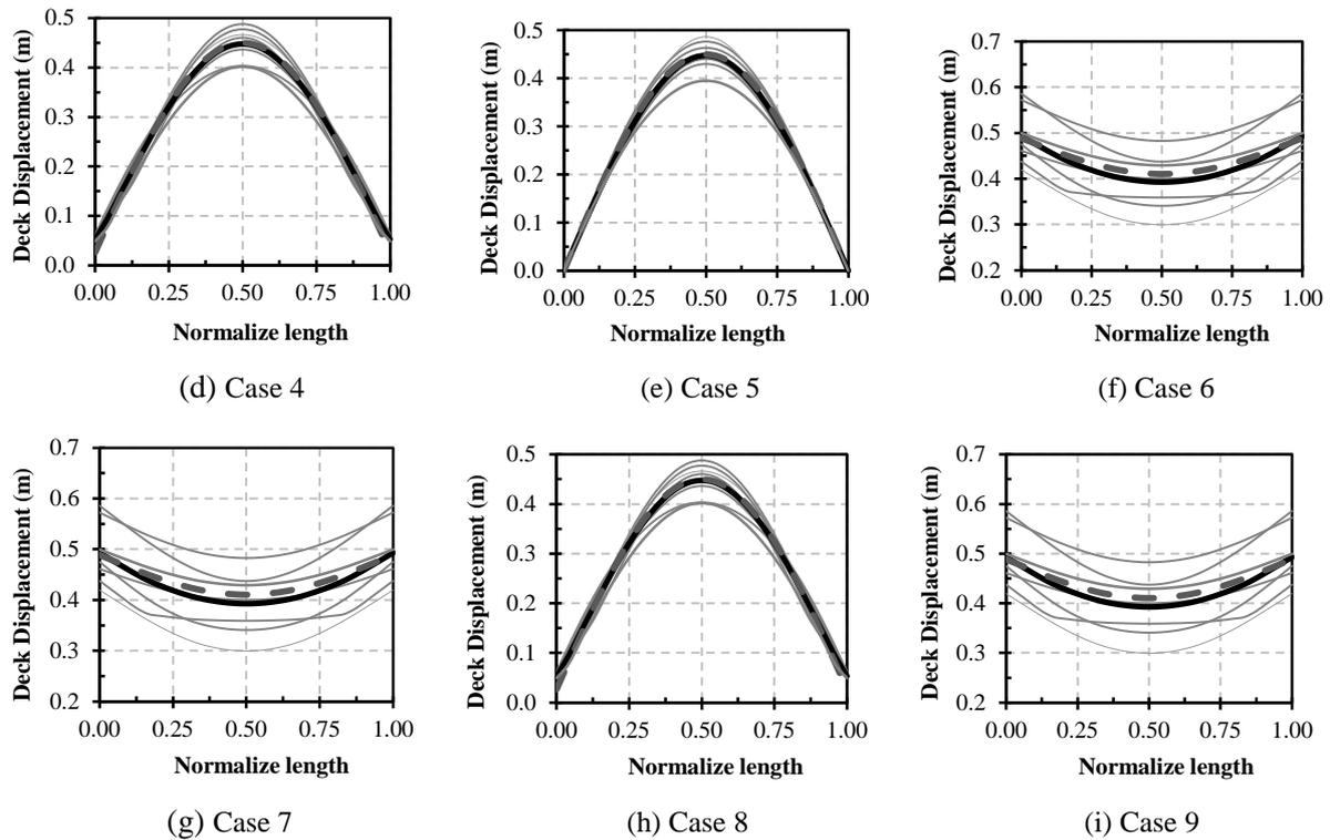
**Figure 3.1** Comparison of ITHA to design target displacements for straight bridges
