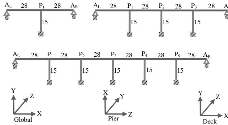
**Figure 2.1** Typical configurations of 2, 4, and 6 span equivalent straight bridges
