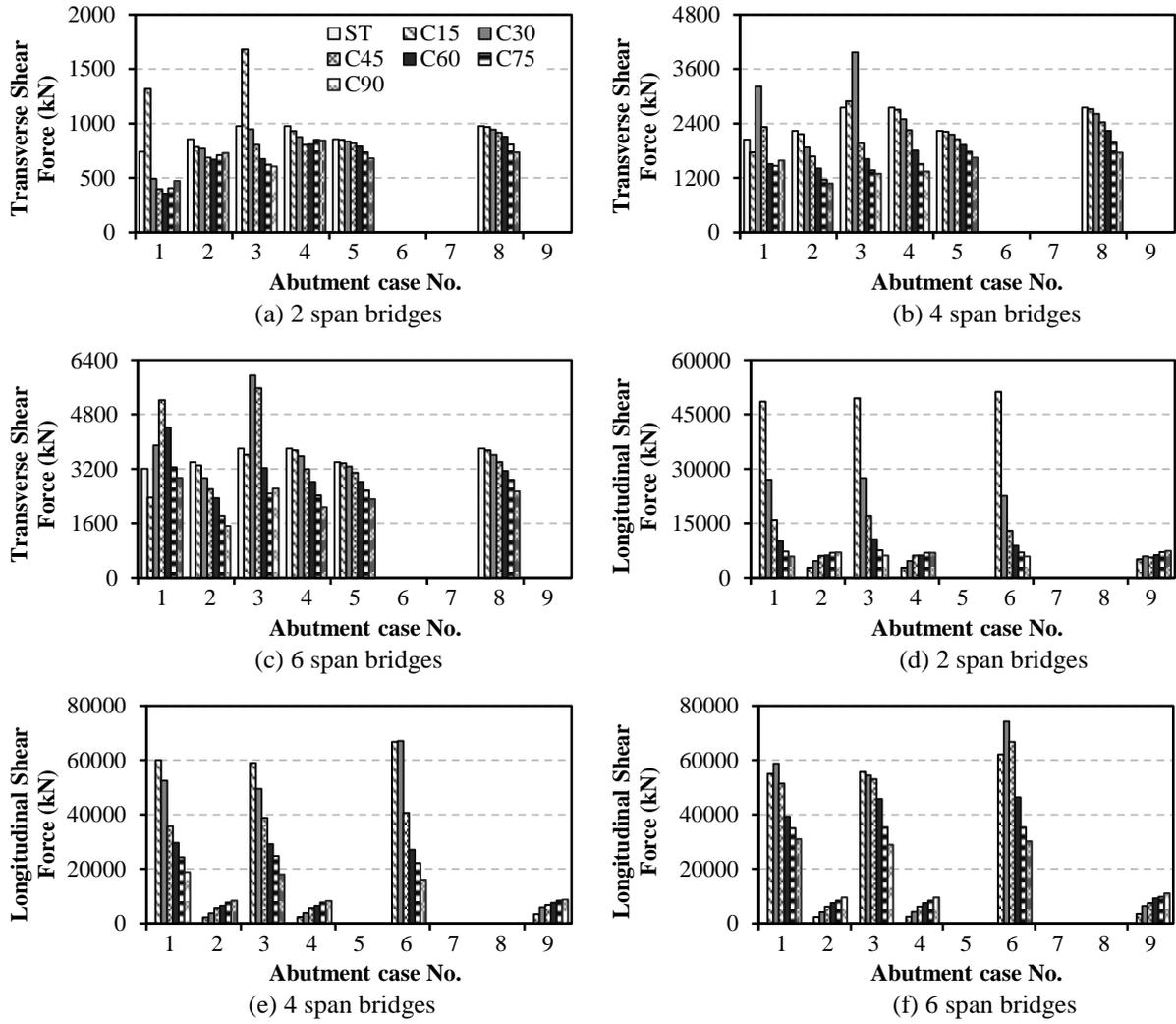
Figure 3.3 Comparison of the ITHA average results of equivalent straight and curved bridges
