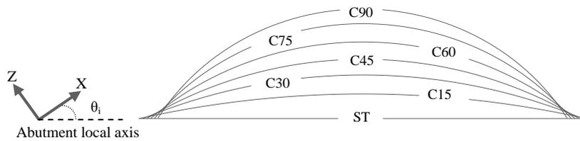
**Figure 2.2** Plane view of straight and curved bridge with different subtended angles
