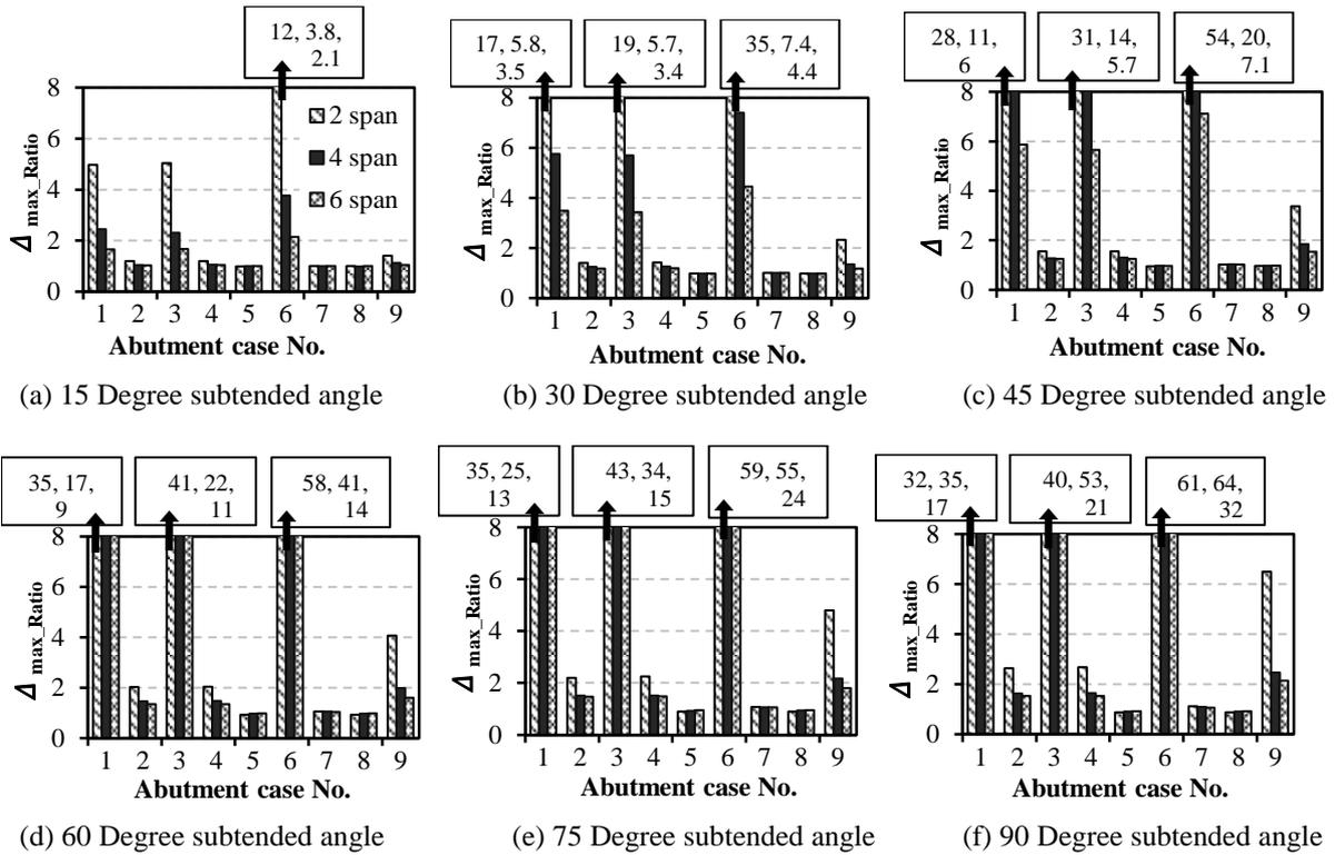
Fig. 3.5 Maximum displacement ratios of the straight to curved bridges grouped by subtended angles
