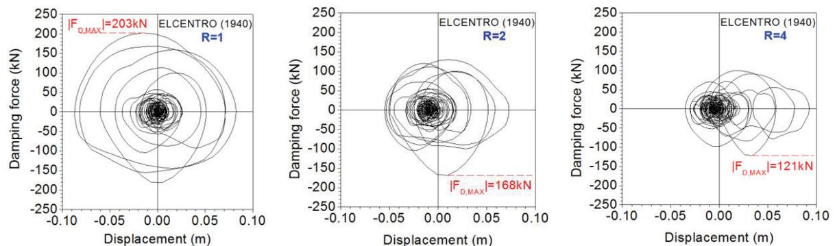
**Figure 3.** Damping force - displacement diagrams for  $R=1, 2$  and  $4$
