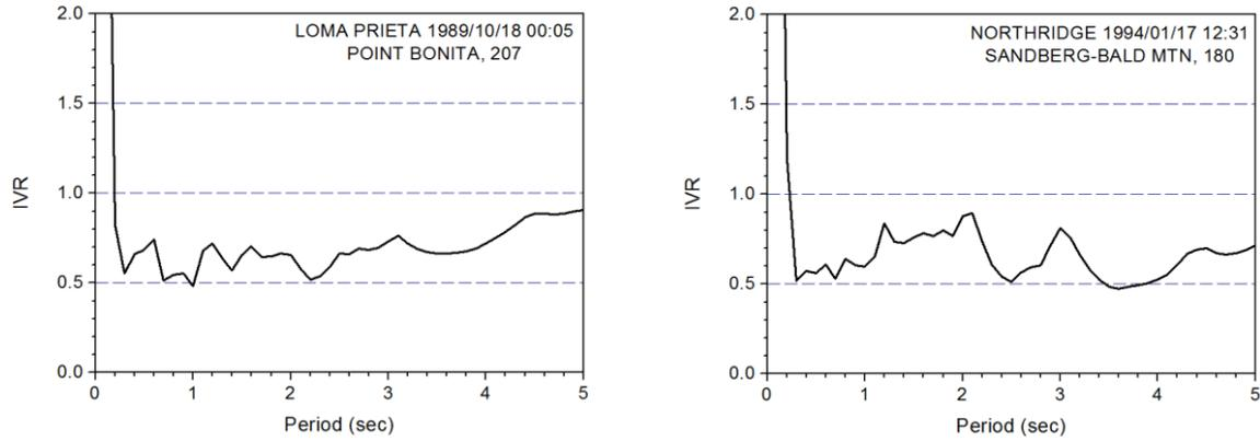
**Figure 1.** Inelastic velocity ratio for characteristic strong ground motions and for  $R=4$ .
