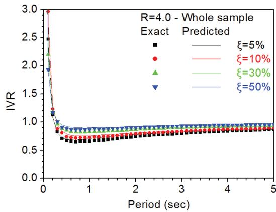
**Figure 5.** Influence of viscous damping on *IVR*
