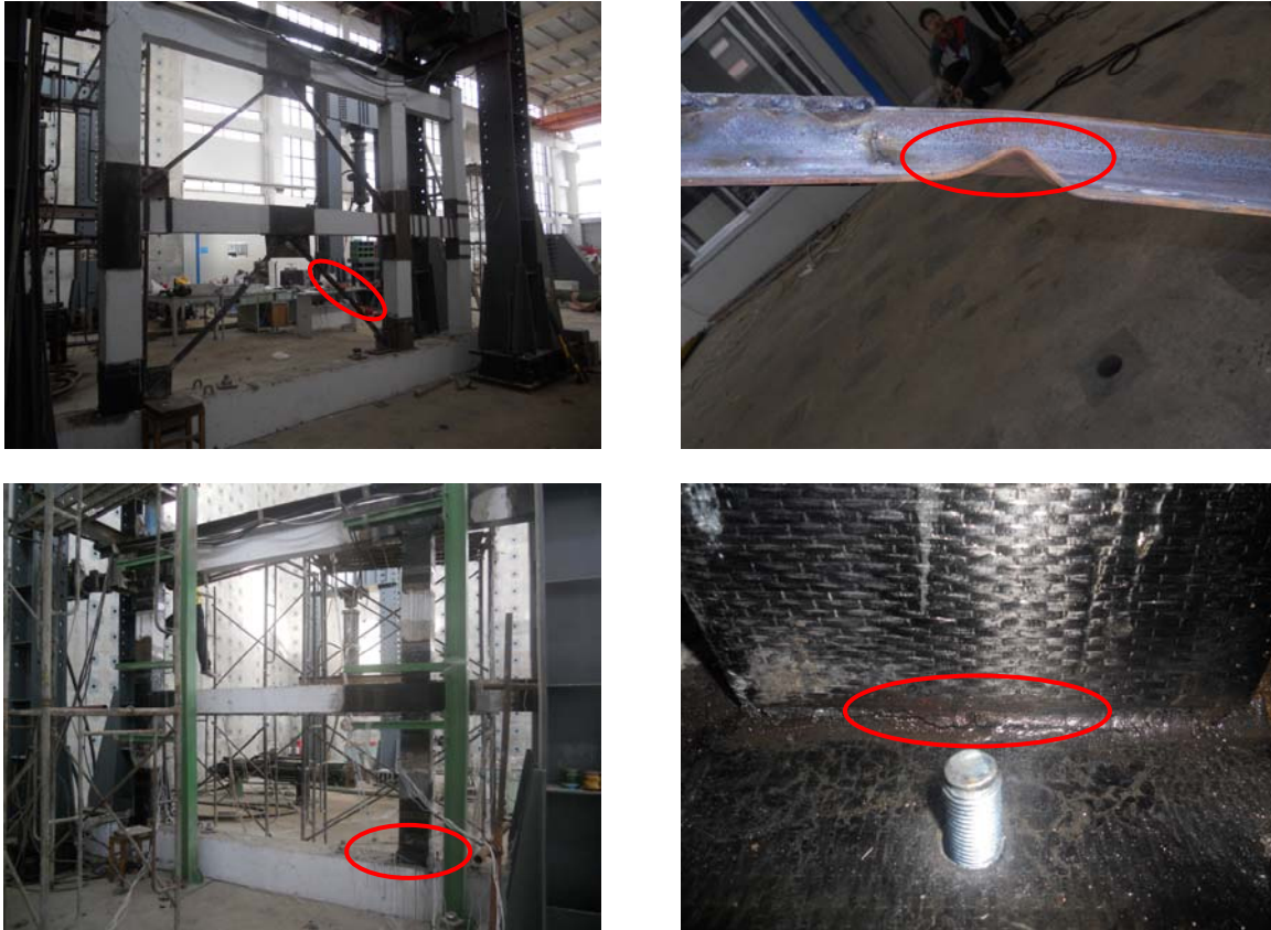
Figure 6. The failure mode of steel brace (a) and FRP (b) retrofitted frames
