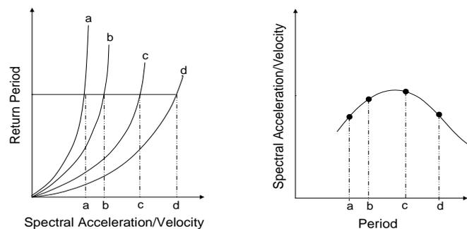
**Figure 5.** Construction of UHRS
