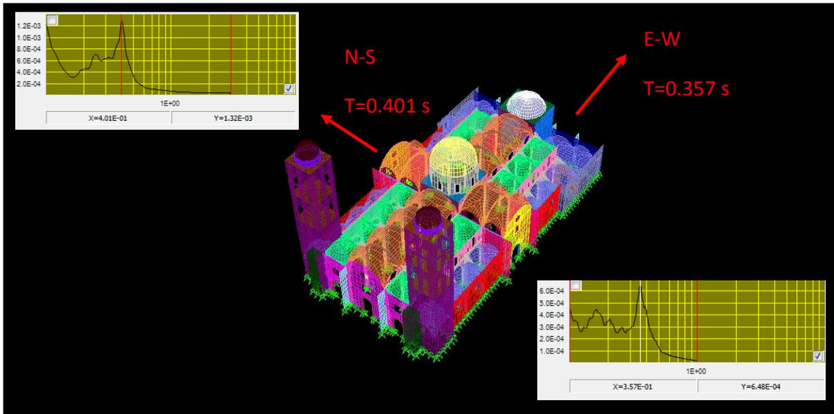
**Figure 5.** Periods of the nave obtained from response spectrums
