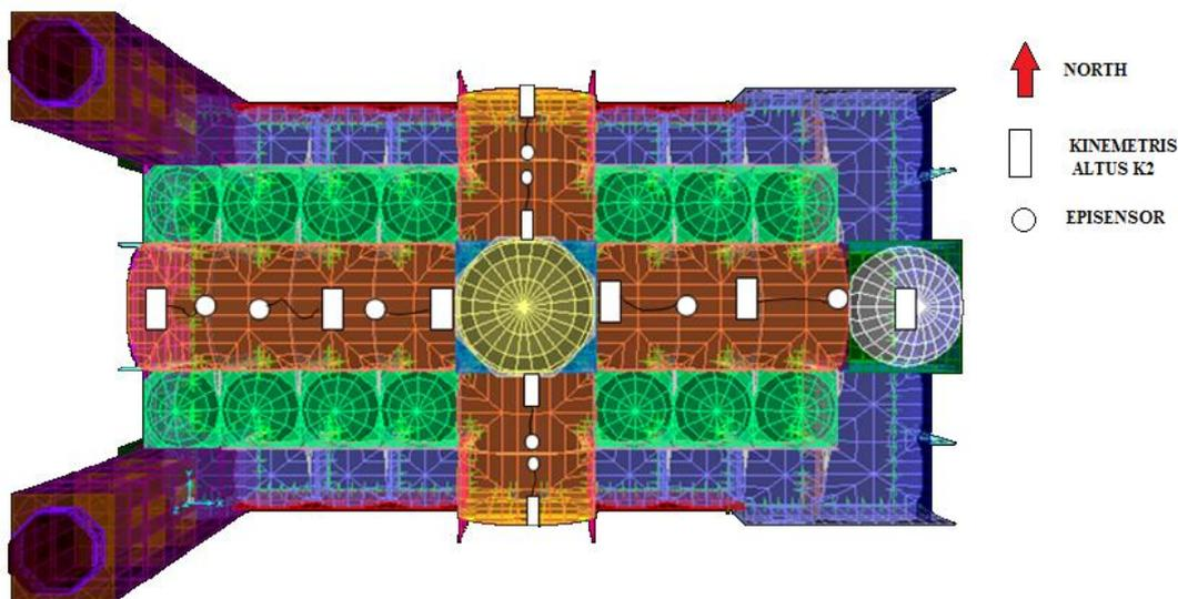
**Figure 3.** Location of the accelerometers on the structure roof
