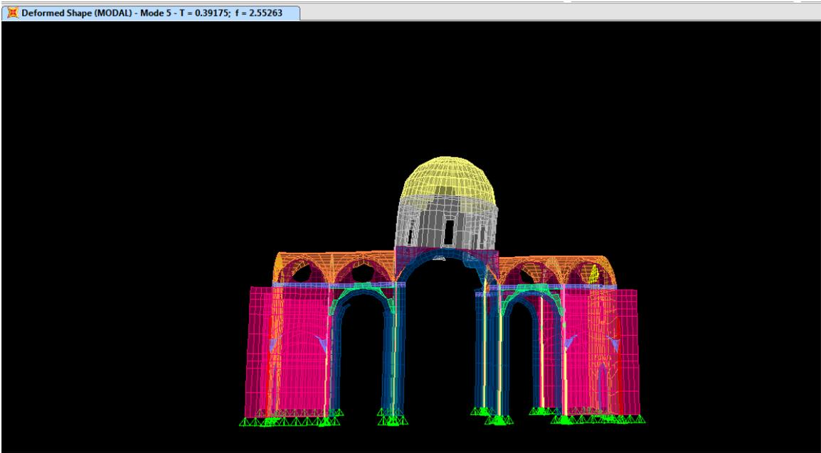
**Figure 6.** Fifth mode. Movement of the nave from North to South
