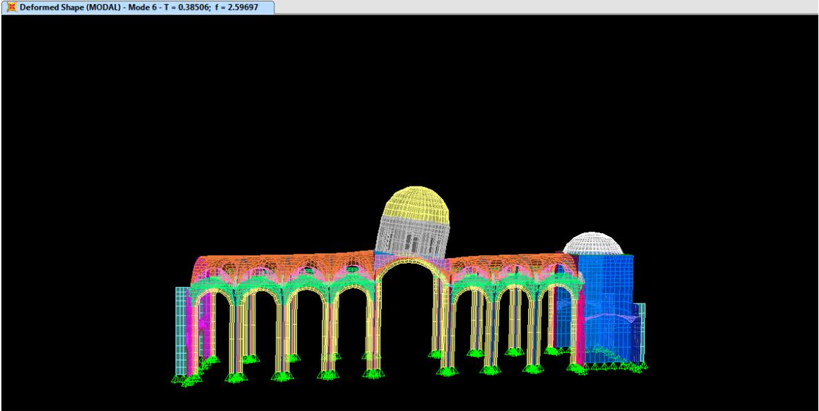
**Figure 7.** Sixth mode. Movement of the nave from East to West
