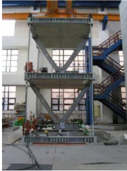
Photo 1. The shaking table test for DSHD with Autonomous Controller
