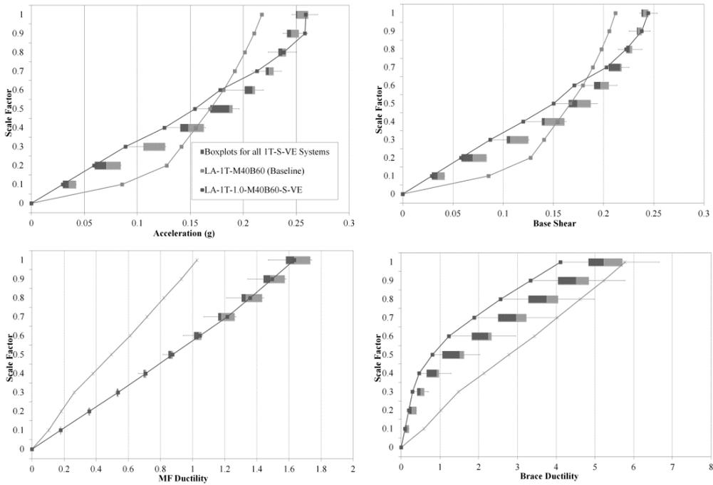
**Figure 4.4.** Identification of the Better Performing Systems
