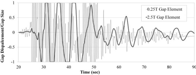
Figure 4.3. Natural Period Comparison of Gap Elements
