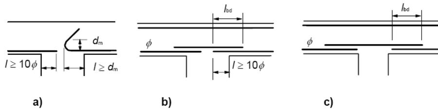
**Figure 9.4: Anchorage at intermediate supports**
