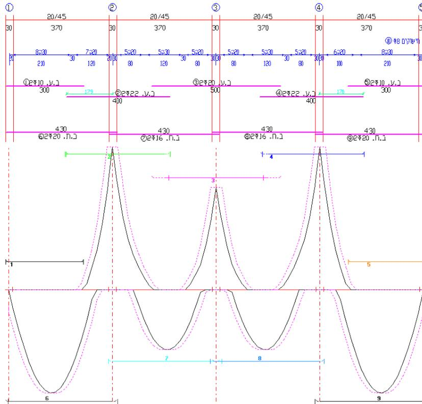
**Figure3.** Example for beam reinforcement detailing without curtailment
