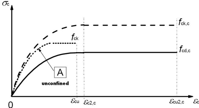
**Figure6.** Stress-strain relationship for confined concrete Euro code 2 [EC2, 2004]
