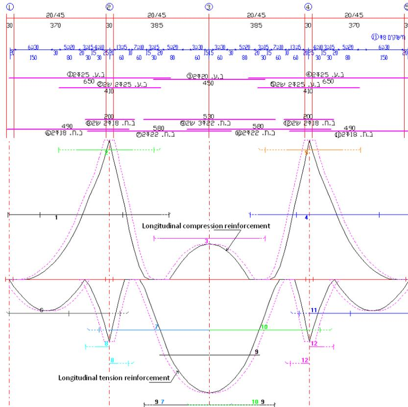
**Figure 4.** Example for beam reinforcement detailing after an interior support removal
