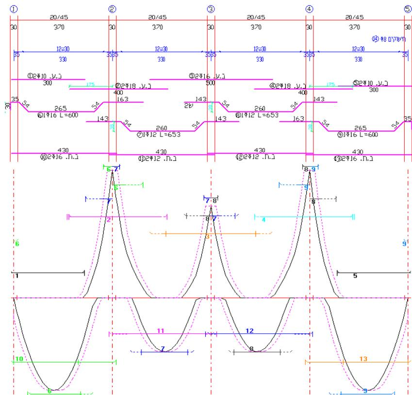
**Figure2. Example for beam reinforcement detailing with curtailment**
