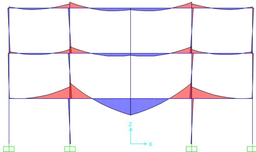
**Figure7.** Bridging over injured zone, interior support elimination, by increasing beam dimensions
