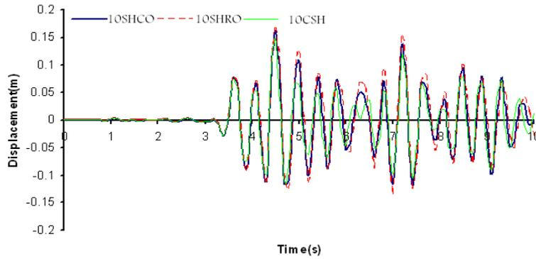
**Figure 6:** Time history of displacements under Taiwan earthquake
