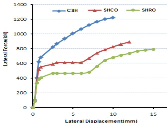
Figure 14. Comparison the Load Paths of the three panel models under lateral loads
