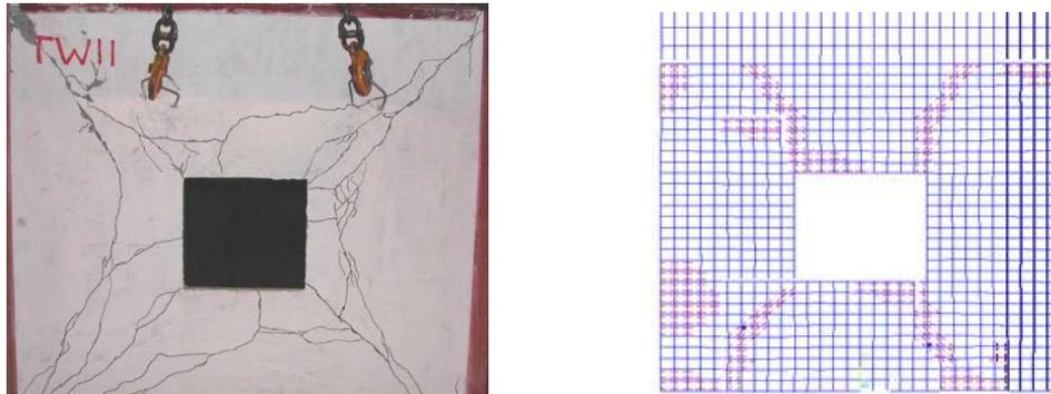
**Figure 10.** Experimental shear wall and ANSYS results
