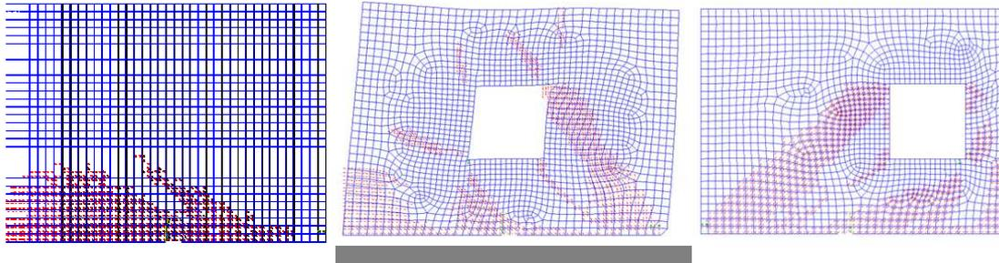
Figure 12. Crack patterns of the three analysed panel models
