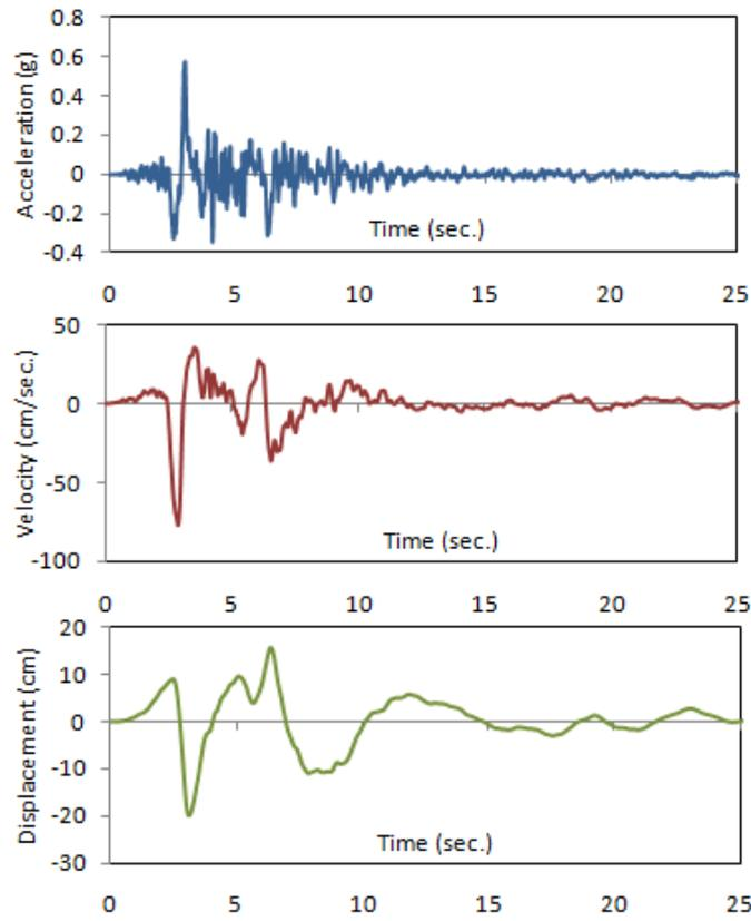
**Figure 2.** Time history components of full record and equivalent pulse. Records obtained from the 1994 Northridge earthquake NGA database.
