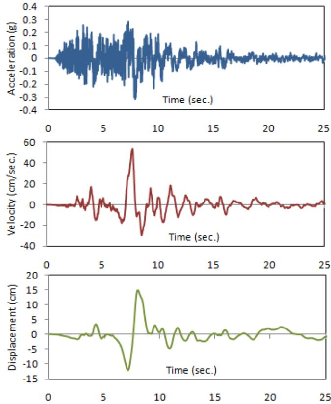
**Figure 4.** Time history components of full record and equivalent pulse. Records obtained from the 1979 Imperial Valley earthquake NGA database.
