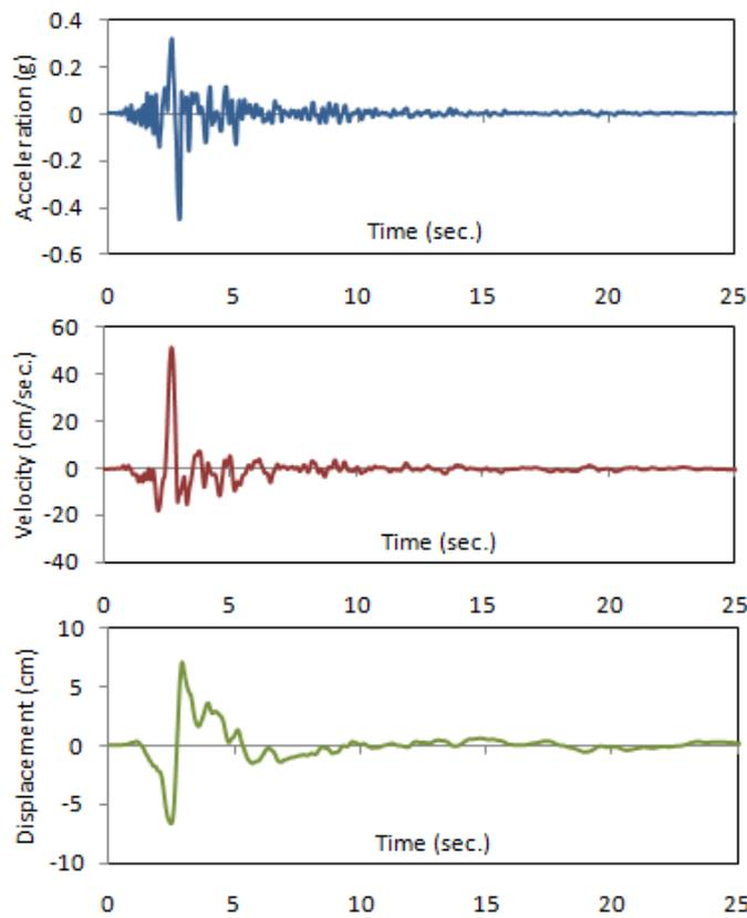
**Figure 3.** Time history components of full record and equivalent pulse. Records obtained from the 1979 Coyote Lake earthquake NGA database.
