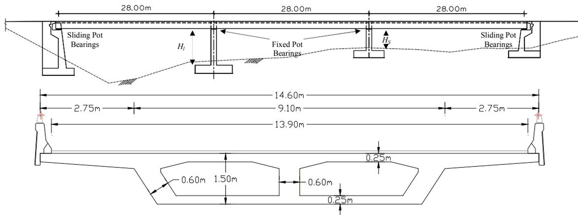
**Figure 3.1.** General arrangement and typical cross-section for the case-study bridge.
