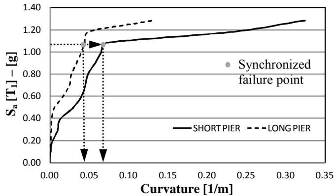
**Figure 6.3.**  $S_a[T_1]$  versus Curvature for bridge long and short piers, case of ratio between piers heights of 0.75 (LP89HDA record).
