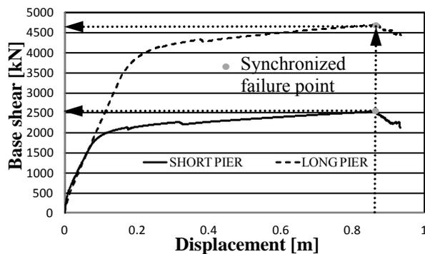
**Figure 6.1.** Base shear-Displacement curve showing synchronized failure of bridge piers for ratio between piers heights of 0.75 – pushover analysis results.
