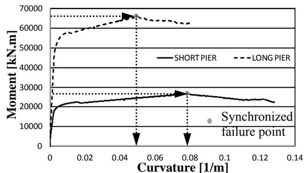
**Figure 6.2.** Moment-Curvature curve showing synchronized failure of bridge piers for case of ratio between piers heights of 0.75 – pushover analysis results.
