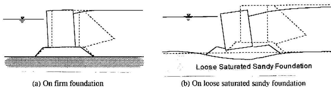
**Figure 1 Deformation/failure modes of gravity quay wall**
