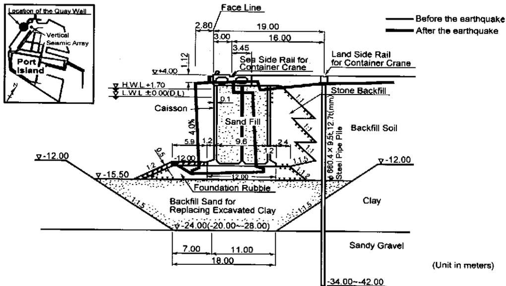
**Figure 2** Location, cross section and residual deformation of a caisson quay wall at Port Island, Kobe Port during Hyogoken-Nambu earthquake of 1995
