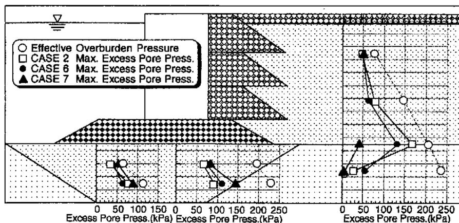
Figure 8 Distribution of maximum excess pore water pressures obtained from shake table tests (scaled in terms of prototype)
