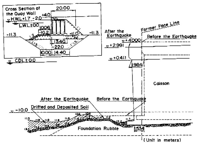
Figure 6 Deformation of rubble mound beneath the caisson (measured by diving)
