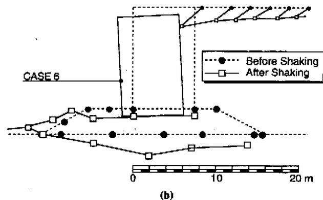
Figure 5 Residual displacement of model quay walls (scaled in terms of prototype)
