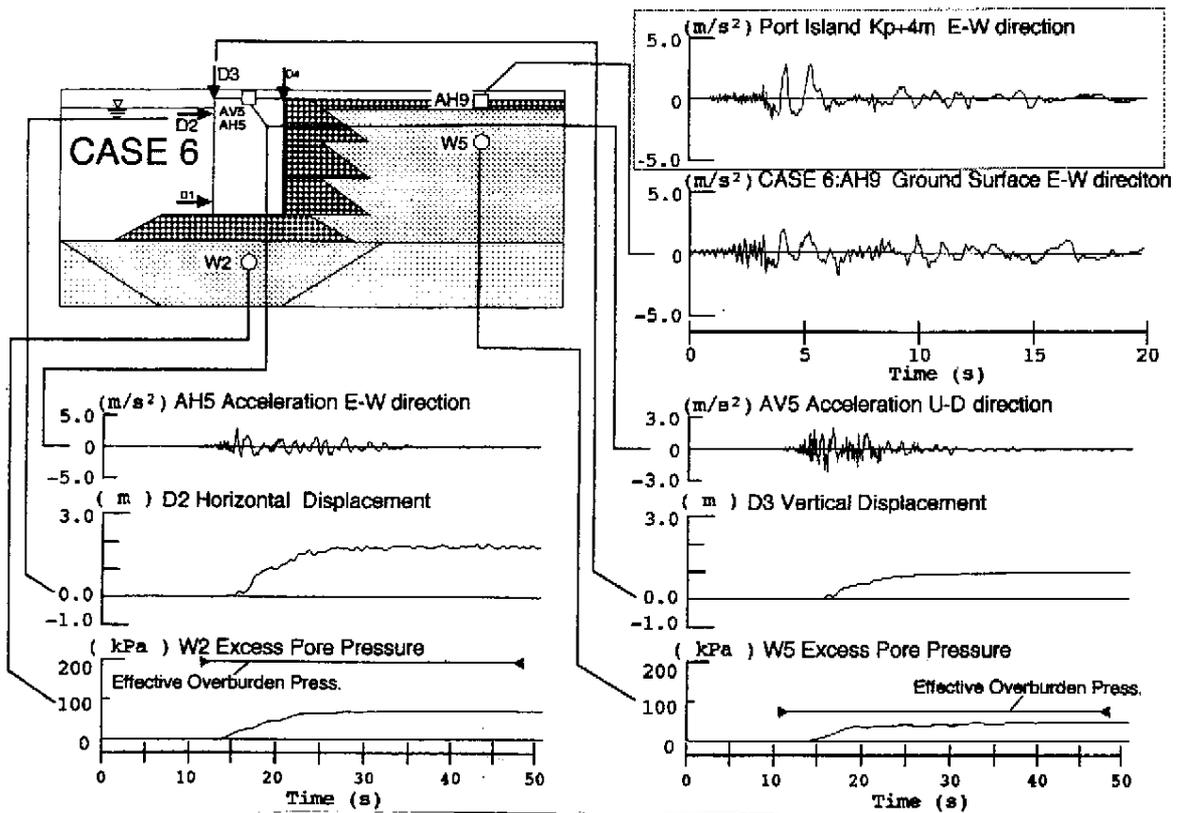
Figure 7 Time histories of model quay wall response (scaled in terms of prototype) and the recorded time history of acceleration at the ground surface at the vertical seismic array site in Port Island
