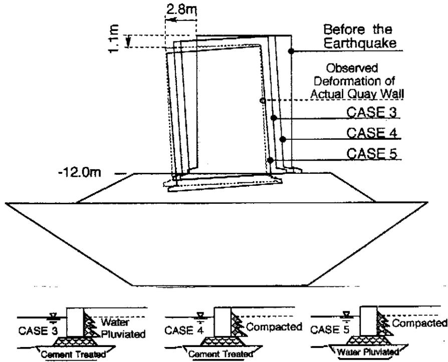
**(b) Displacements of caisson wall (Cases 3 through 5)**
