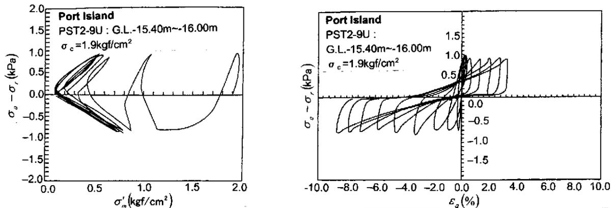
**Figure 3** Undrained triaxial tests results of in-situ frozen sample of foundation soil at Port Island
