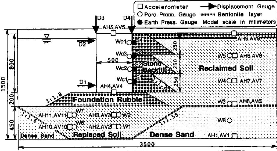
Figure 4 Cross section of a model quay wall for shaking table tests
