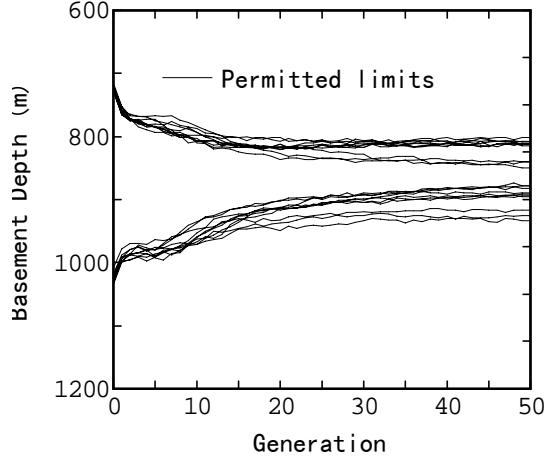
**Figure 10: Permitted limits of basement depth in the inversion at Tomioka site**
