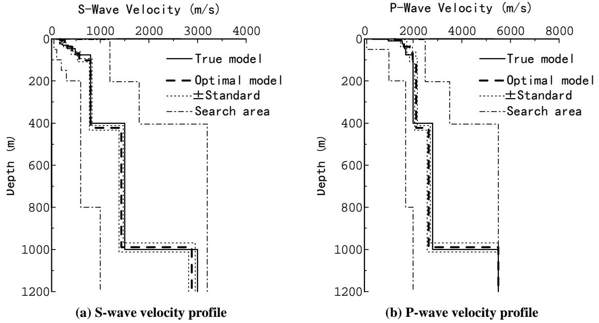
**Figure 4: Comparison of the optimal model from model B inversion with the true model**
