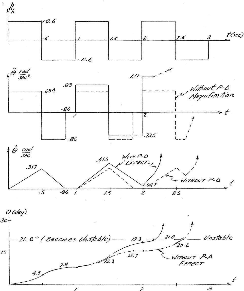
**Figure 4. Integration of Angular Deformation of Retaining Wall with Bearing Capacity Failure. APPLICATION TO KOBE WALL**
