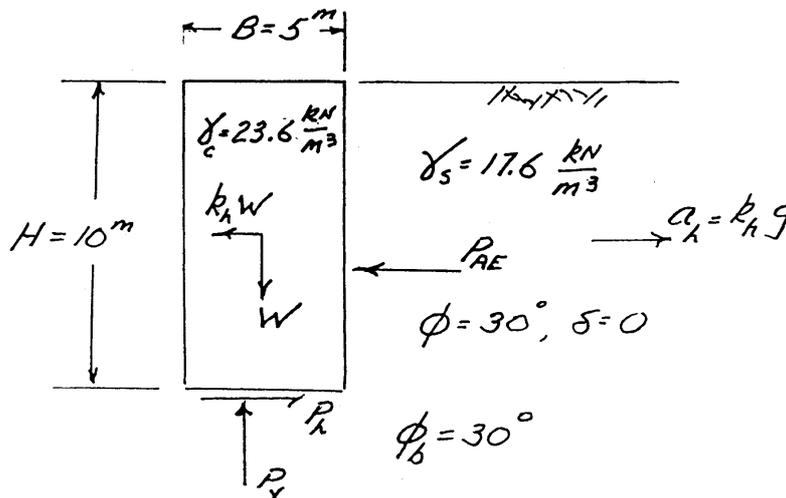
Figure 2. Retaining Wall for Simple Example Problem
