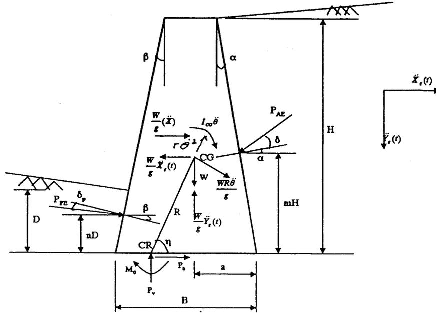
Figure 1. Free Body Diagram of Retaining Wall
