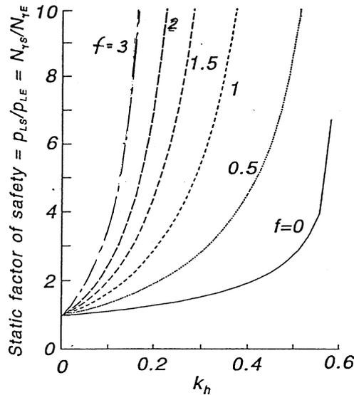
Figure 3. Bearing Capacity Factors for  $\phi_b = 30^\circ$
