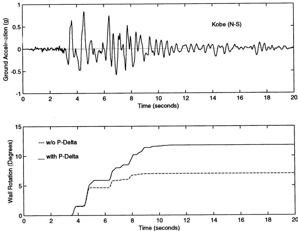
Figure 6. Kobe 1995 Earthquake, N-S Component Acceleration Time History and the Rotational Response of the Example Retaining Wall
