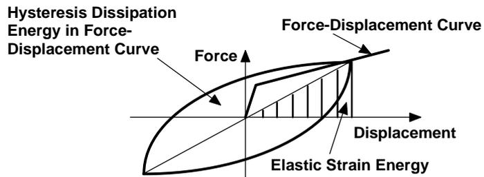
(b) Energy for Equivalent Damping Ratio
