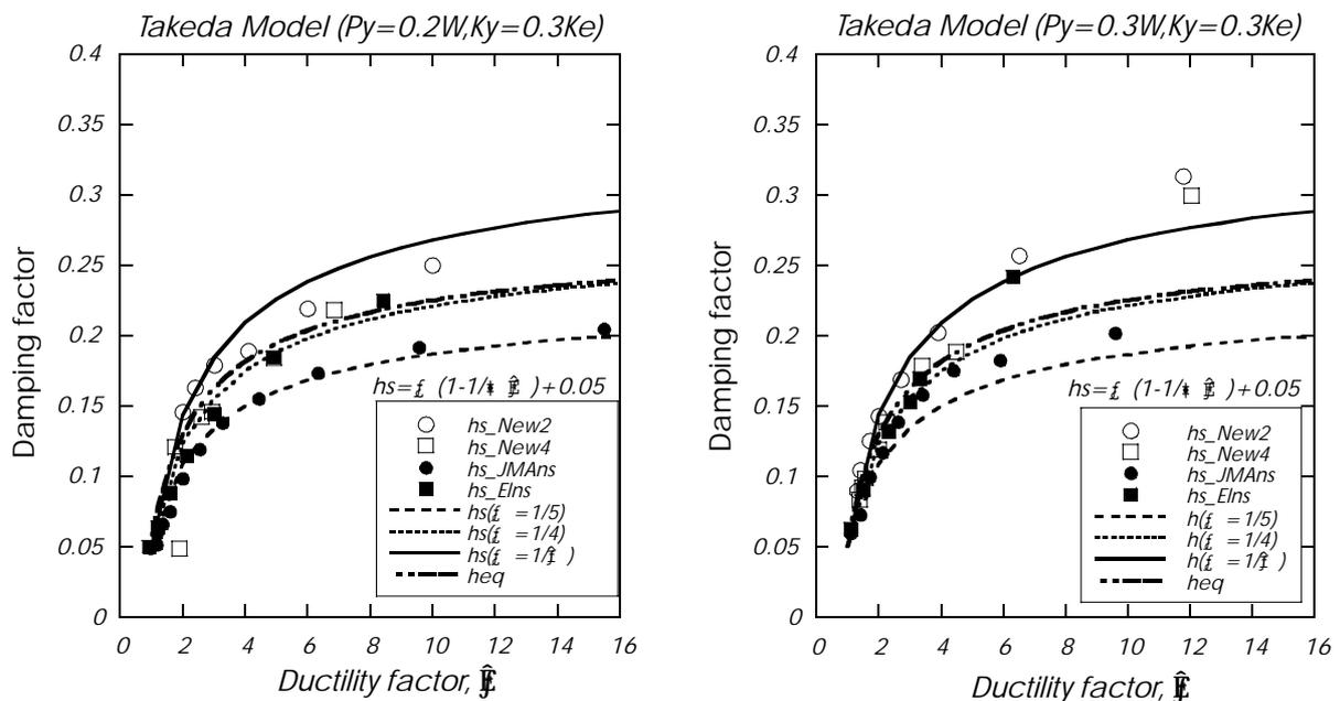
Fig. 3 (a) Damping factor for RC members
