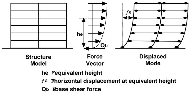
(a) Structure Model and Inelastic Response
