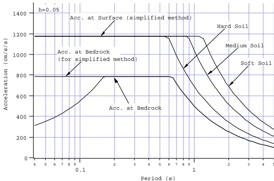
**Fig.1 Acceleration response spectrum at engineering bed rock and surface**
