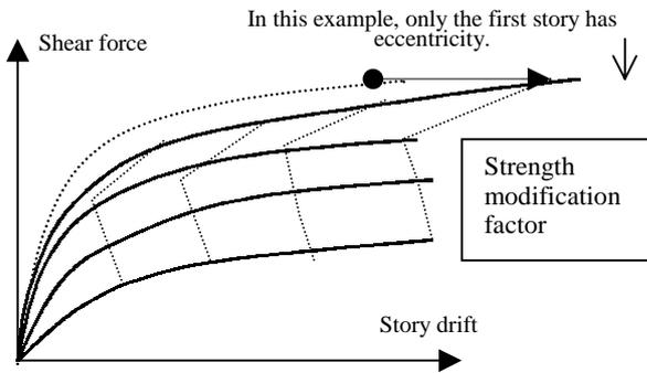
**STEP3:** In order to predict story drifts at the perimeters in the damage-predicted sides, amplify the values predicted in STEP2 for the story drifts near the center of gravity by the deformation amplification factor.
