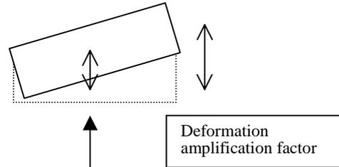
The horizontal seismic design force distribution is supposed to be unchanged still after decreasing the strength capacities. Then story drift distribution can be computed without redoing pushover analysis.
