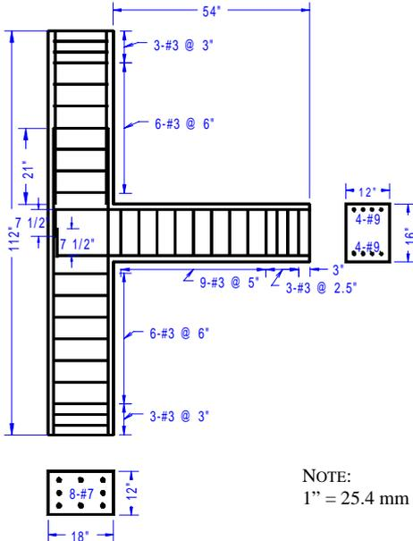
**Figure 1. Specimen dimensions and reinforcement details**
