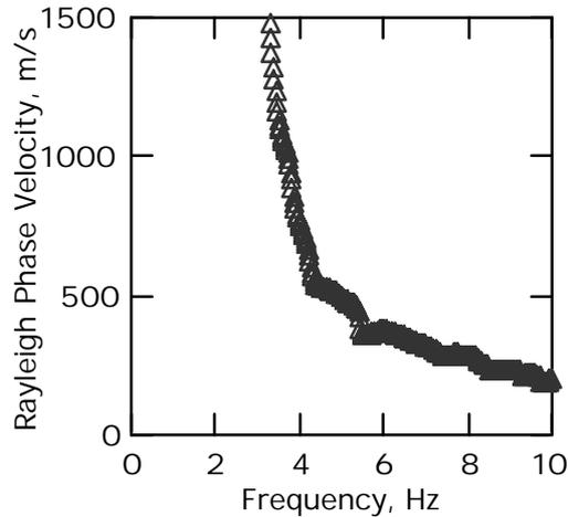
**Figure 3:** Estimated phase velocities of Rayleigh wave from vertical components of microtremors at the site of Nioh elementary school. The Rayleigh wave phase velocities are used to estimate Love wave phase velocities from horizontal components of microtremors using spatial auto-correlation method.
