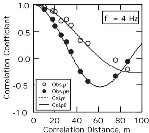
**Figure 5:** Comparison with observed values of correlation coefficients and calculated values for the Nioh site at a frequency of 4 Hz. Open circles mean radial components of observed correlation coefficients and solid circles mean tangential components of observed correlation coefficients. Dashed line means radial components of calculated correlation coefficients and solid line means tangential components of calculated correlation coefficients.
