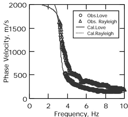
**Figure 7:** Comparison with observed values of phase velocities and theoretical values at the Nioh site. Triangles mean observed phase velocities of Rayleigh wave and circles mean observed phase velocities of Love wave. Dashed line means theoretical phase velocities of Rayleigh wave and solid line means theoretical phase velocities of Love wave. Theoretical phase velocities were calculated from S-wave velocity structure shown in Table 1.
