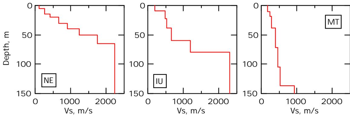
**Figure 9:** Estimated S-wave velocity structure models at three experimental sites at a function of depth. See the caption of Fig. 8.
