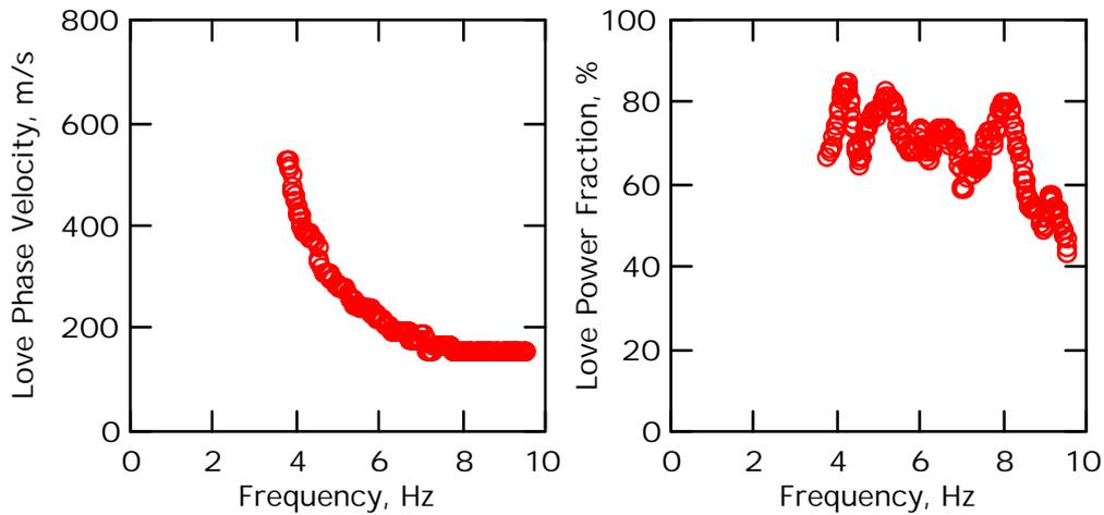
**Figure 6:** Estimated phase velocities of Love wave from horizontal components of microtremors using phase velocities of Rayleigh wave shown in Fig. 3 (left). Estimated power fraction of Love wave in microtremors (right). The power fraction of Love wave is defined as the ratio of Love wave power and total microtremor power. (4).
