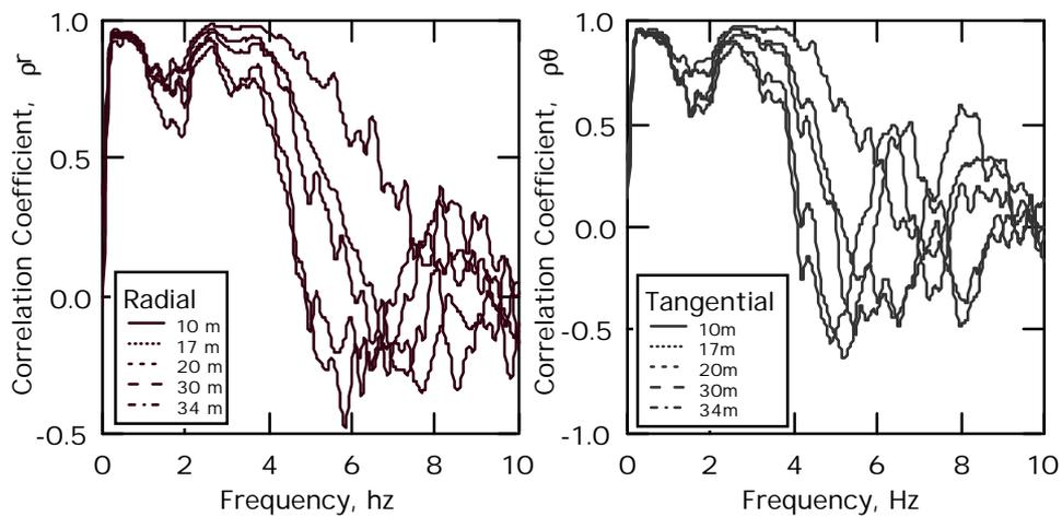
**Figure 4:** Radial components of spatial auto-correlation coefficients as a function of frequency calculated from horizontal microtremor data of R=20m array of Nioh site (left). Legend means correlation distances. From one array observation, we can five kinds of correlation distances. Tangential components of spatial auto-correlation coefficients as a function of frequency calculated from horizontal microtremor data of array of the same site (right).
