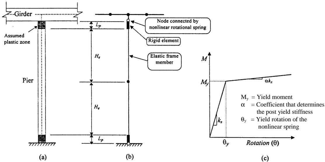
**Fig. 3: Modeling of a pier by an elastic column and nonlinear rotational springs at both ends**
