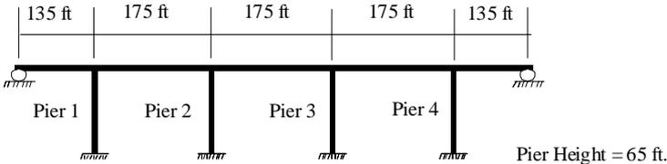
**Fig. 1: Elevation of TYOH Bridge**
