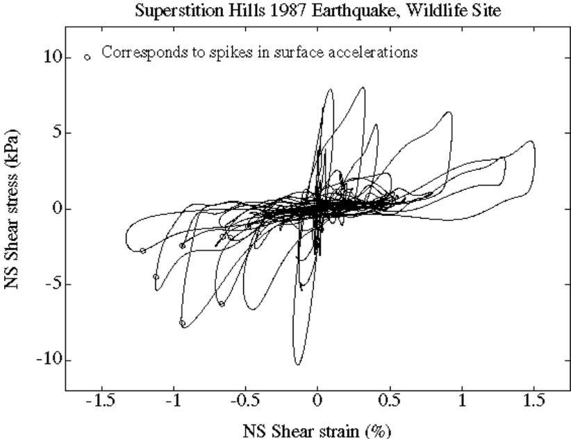
**Figure 4: Wildlife Refuge shear stress-strain response at 3.75 m depth [Zeghal and Elgamal 1994].**
