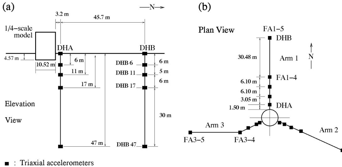
Figure 2: Instrumentation of Lotung experiment site [Tang 1987]: (a) downhole array; (b) surface array.
