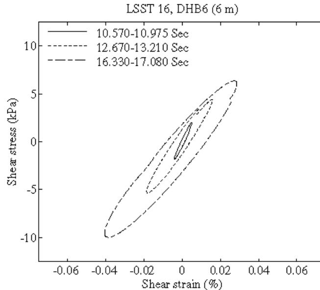
Figure 3: Samples of Lotung site shear stress-strain cycles at 6 m depth [Zeghal *et al.* 1995].
