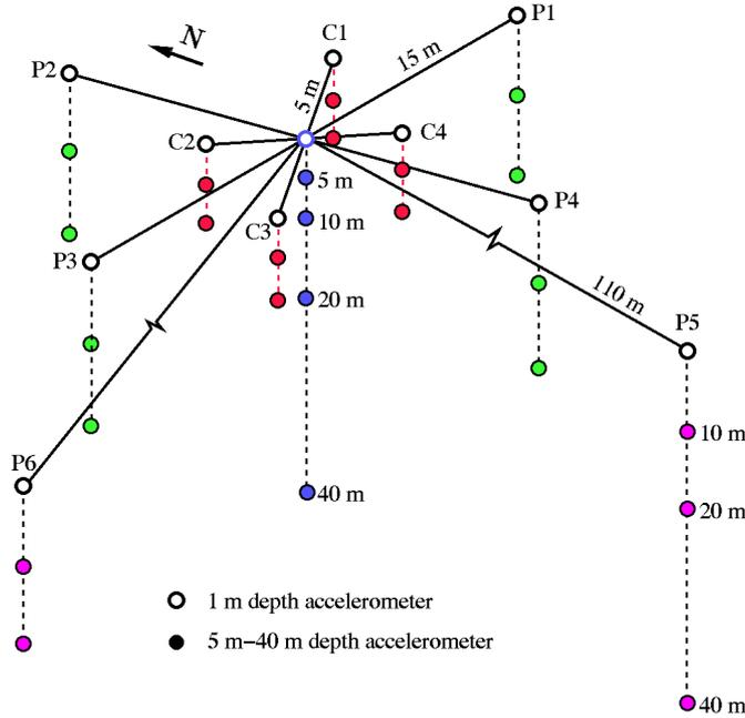
Figure 1: Three-dimensional array at Chiba, Japan [Katayama 1990].
