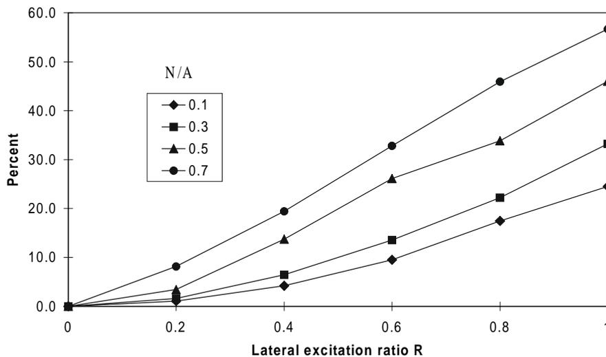
Figure 7 Percentage increase in displacement for  $\mu=0.8$  for different values of  $N/A$
