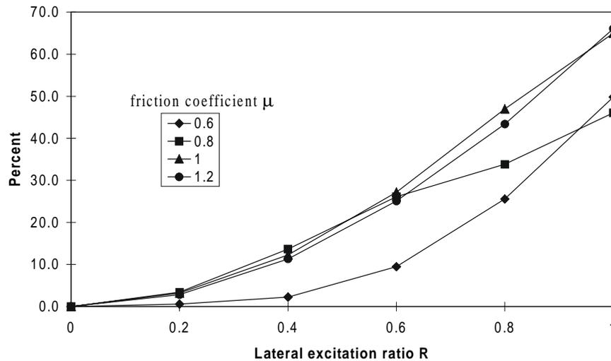
Figure 8 Percentage displacement increase for  $N/A=0.5$ , with different values of  $\mu$
