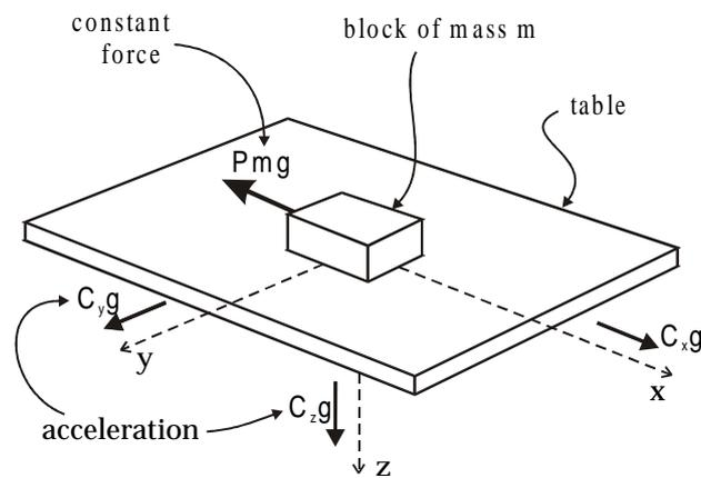
Figure 1 Three-dimensional sliding block model
